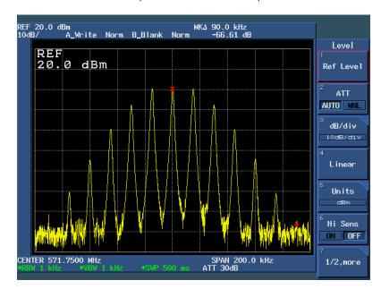
OCCUPIED BANDWIDTH—POWER OUTPUT = 2000 watts Visual, 200 watts Aural (Scan width = 200 kHz)
