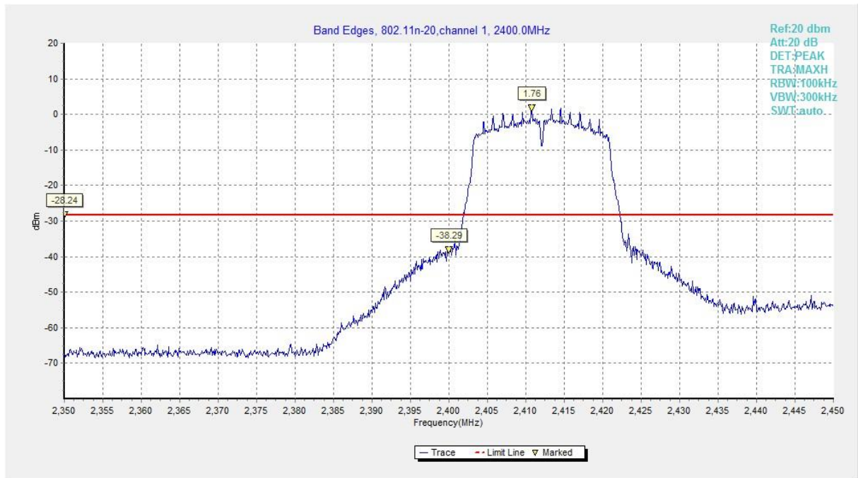
Fig.23 Band Edges (802.11n-HT20, CH 1)
