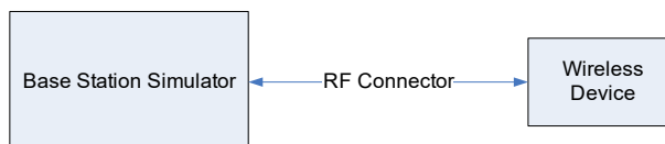
Figure 10-4 Power Measurement Setup – NR FDD
