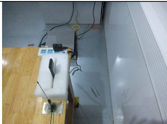
Conducted Emissions Test Setup Side View
