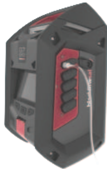
Tubing connected to EXO's manual calibration inlet
