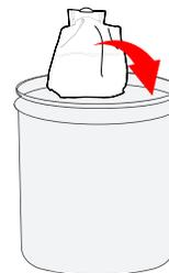
Hold the handle to lift out the dust bag, which can effectively prevent dust leakage.
