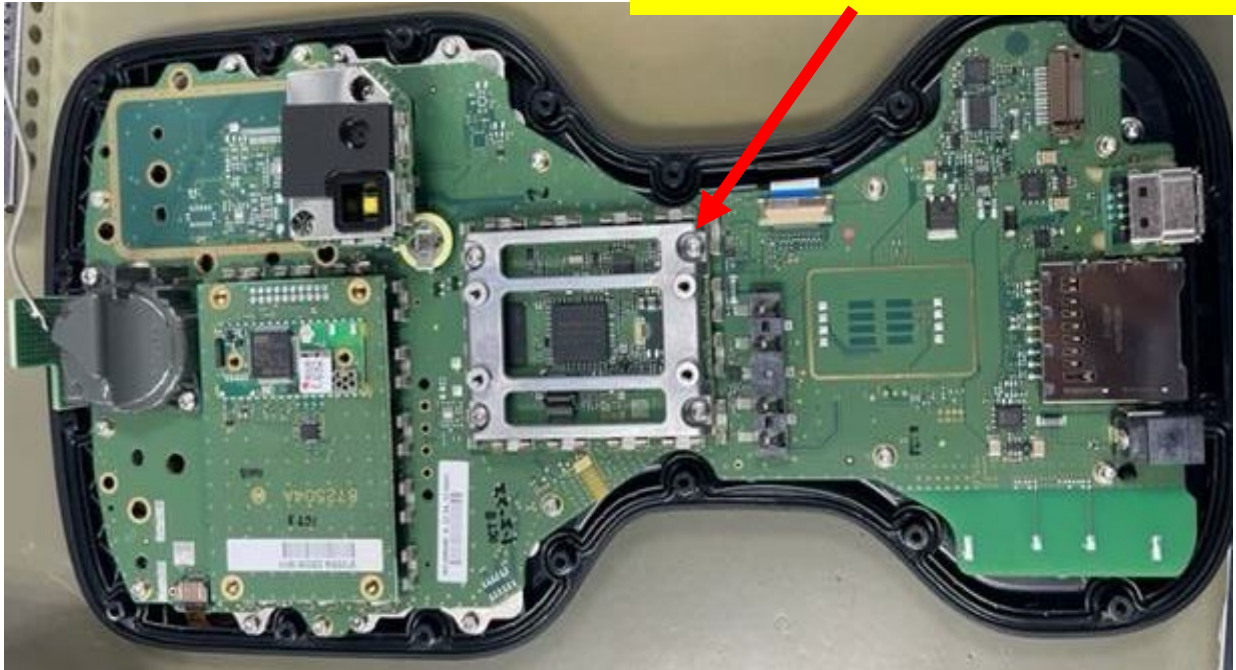
Core Module after casing removed
