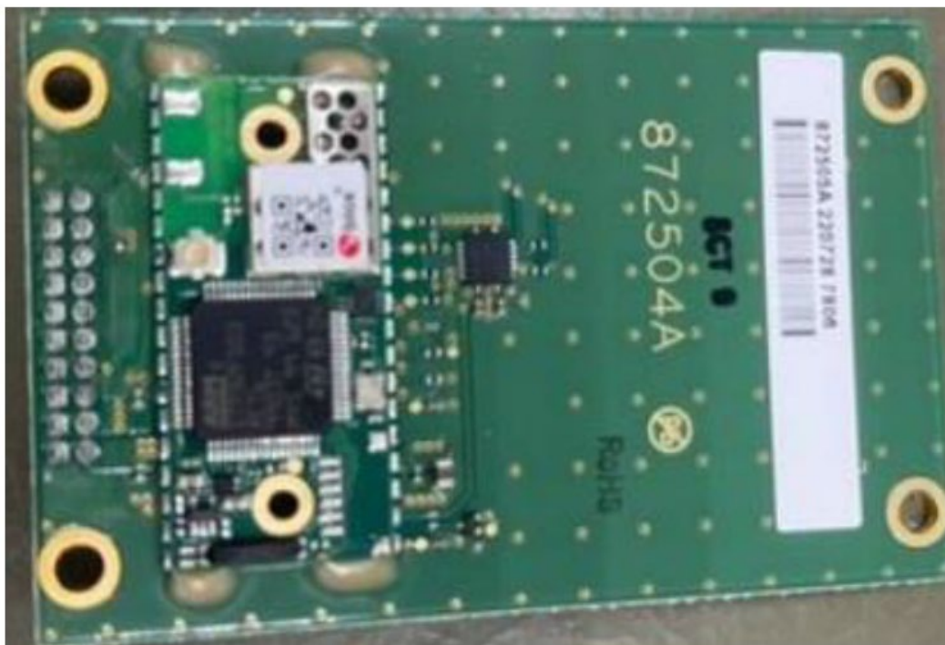
08 EUT PCB LONG-RANGE BLUETOOTH BOARD TOP SIDE
