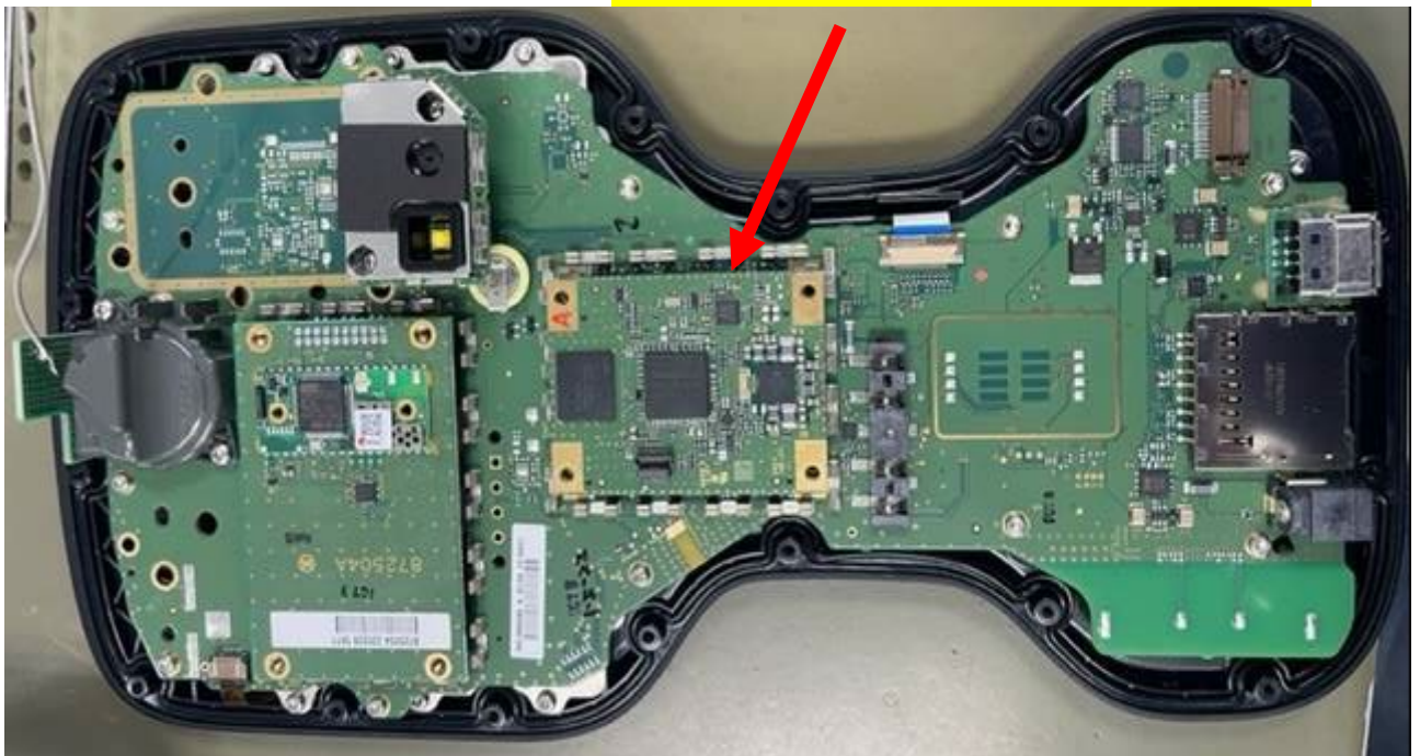
Core Module after casing removed
