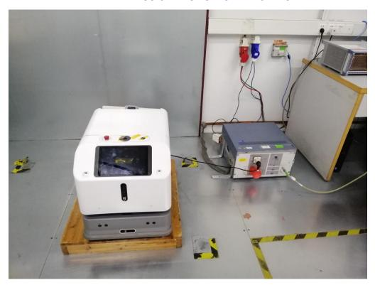
RADIATED EMISSION TEST SETUP ABOVE 1GHz
