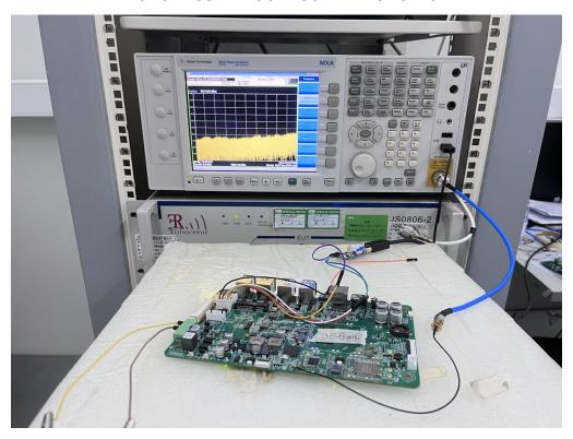
MODULE AP6275 RF CONDUCTED TEST SETUP
