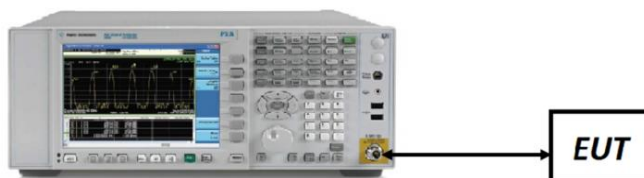
Figure 7-3. Test Instrument & Measurement Setup
