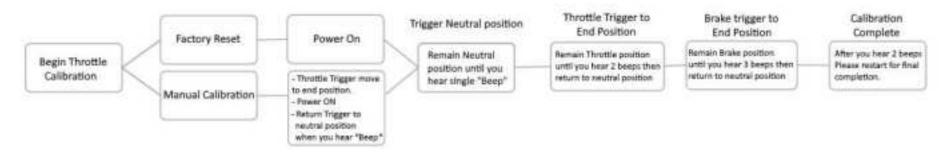
开始油门校准 Start to calibrate the throttle 第一次校准 First calibration 恢复出厂设置后校准 Calibration after restoring factory settings 重新校准 Recalibration
