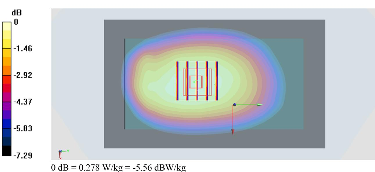
**#20\_LTE Band 17\_10M\_QPSK\_1RB\_0offset\_Back\_10mm\_Ch23790**
