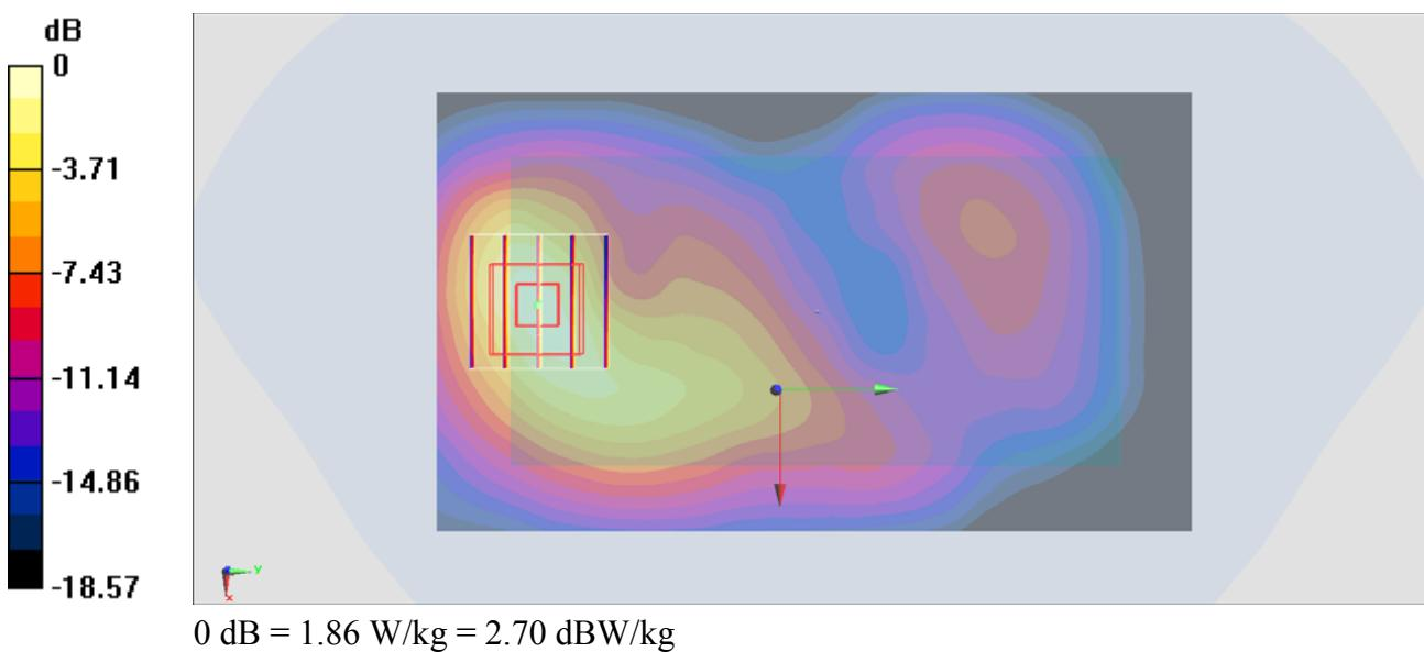
**#32\_LTE Band 12\_10M\_QPSK\_1RB\_0offset\_Back\_10mm\_Ch23095**
