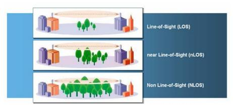
Whereas multi-pathing degrades a link in some technologies (FSK, for example), OFDM can often use multi-pathing to an advantage to overcome nLOS, especially in cases where the Fresnel zone is only partially blocked by buildings, "urban canyons", or foliage. OFDM tends to help especially when obstacles are near the middle of the link, and less so when the obstacles are very near the SM or AP.
