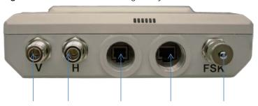
Path V RF Port Path H RF Port Sync/Default Ethernet Unused
