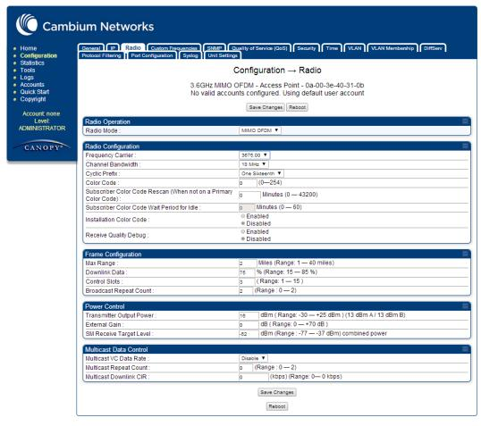
The Radio tab of the AP contains some of the configurable parameters that define how the AP operates.
