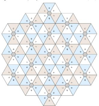
Figure 19 Example layout of 16 Access Point sectors (ABC), 60 degree sectors
