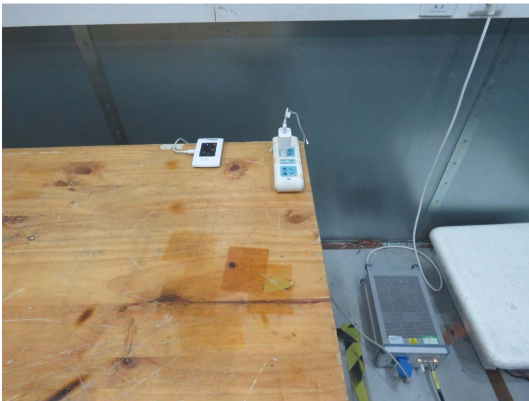
Picture 2 Conducted Emission Test Setup
