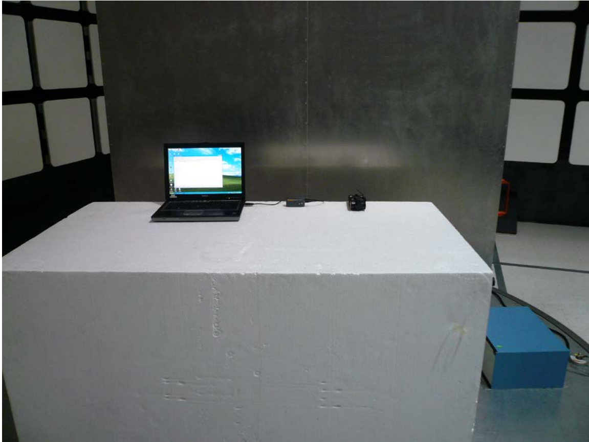
Figure 8: AC Conducted Emission Test Setup (Front)
