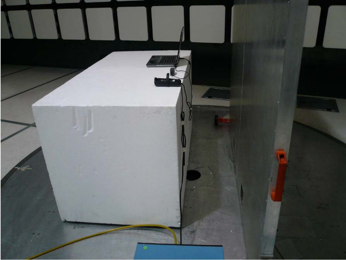
Figure 9: AC Conducted Emission Test Setup (Front)
