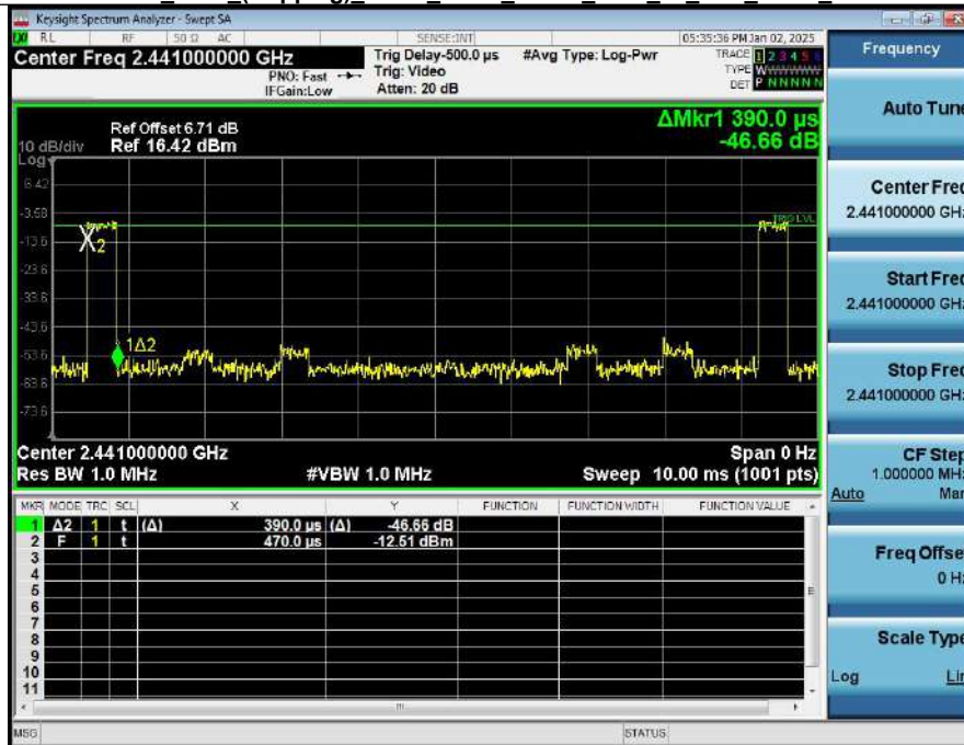
Dwell Time (Hopping) NVNT ANT1 1-DH1 2441 00 Accumulated
