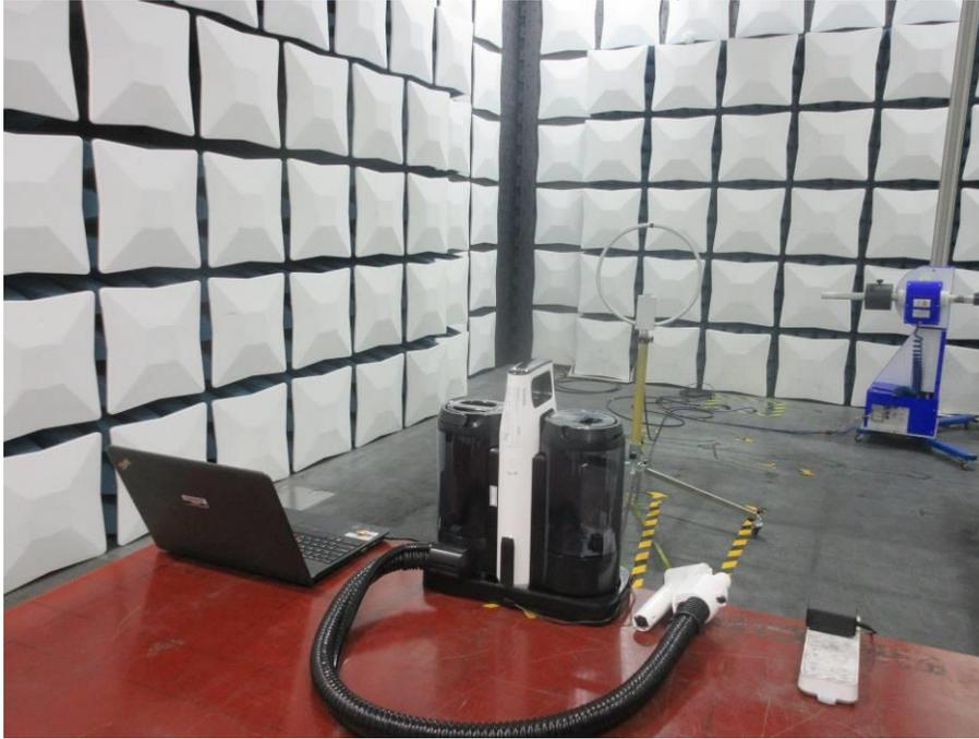
RADIATED RF MEASUREMENT SETUP (30MHz ~ 1 GHz)
