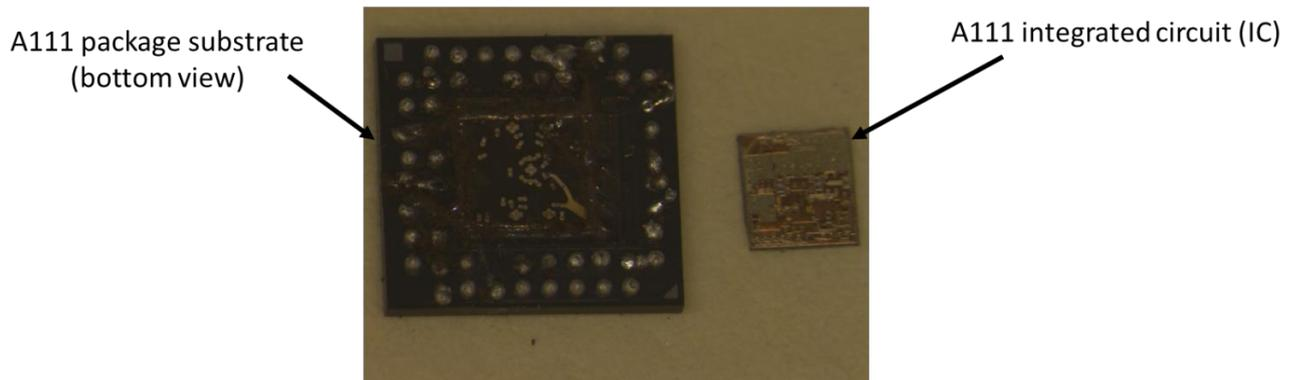
External pictures: A111 radar sensor - top and bottom view:
