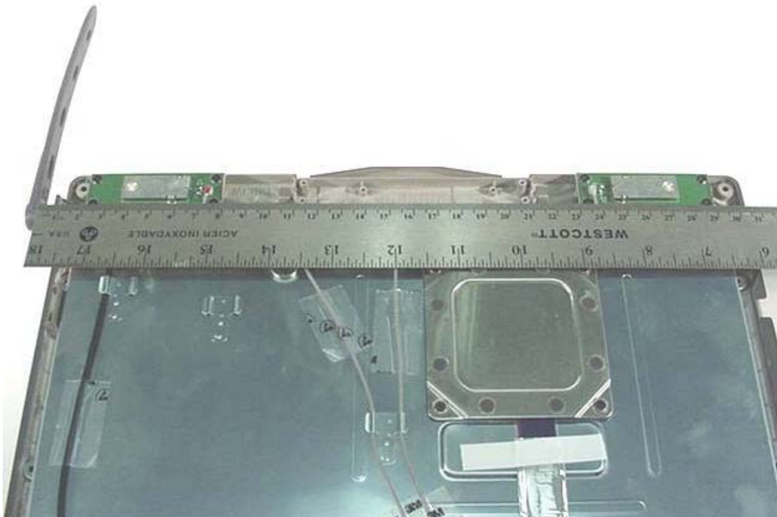
Distance at LCD back-side between dipole antenna feed/swivel-joint and WLAN dual antennas
