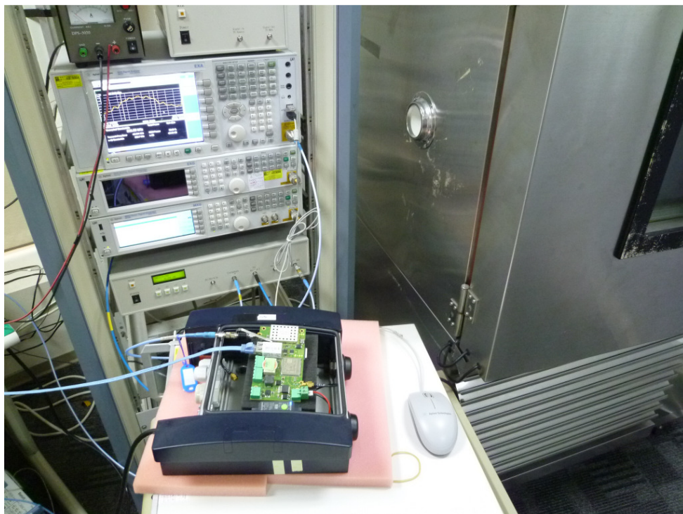
Photograph 4: Set-up for Conducted testing
