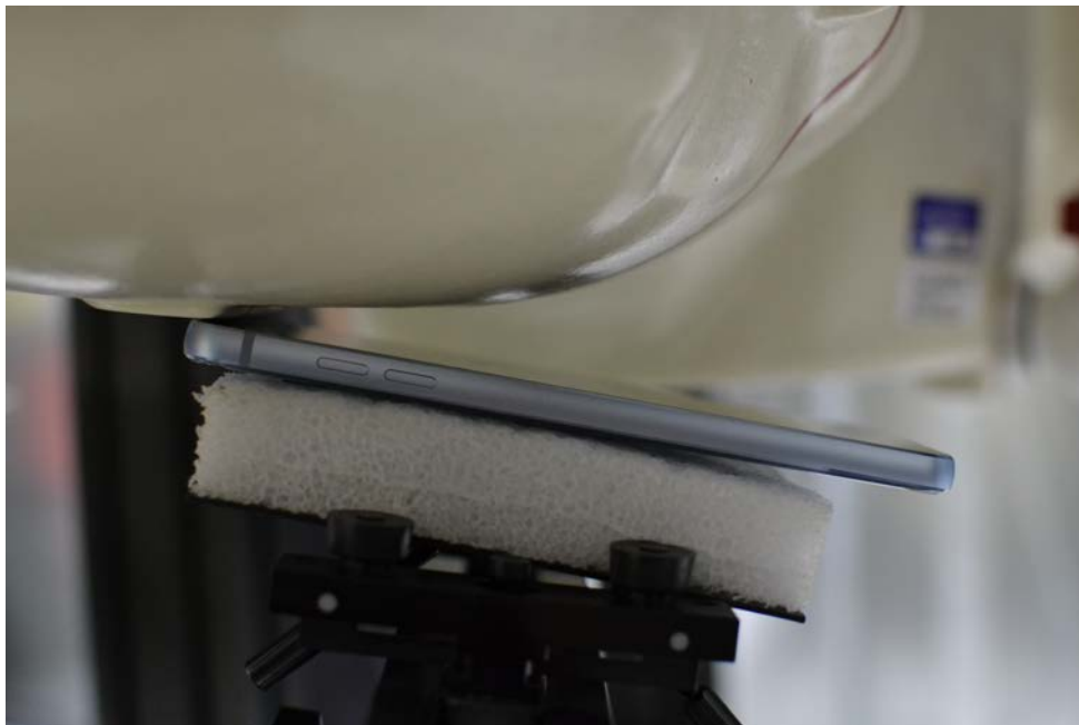
SAR Test Setup Photo 2: Right Tilt
