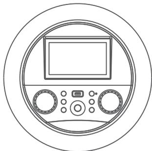
The TFT touch screen will be switched on automatically when the unit is powered on.
