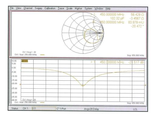
Impedance Measurement Plot for Head TSL
