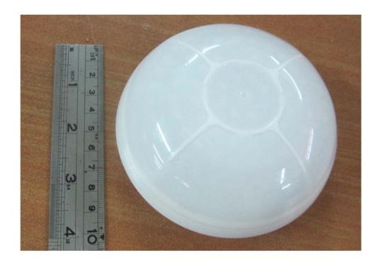
Photograph No.2 PG9862 PIR presence/security detector rear side view
