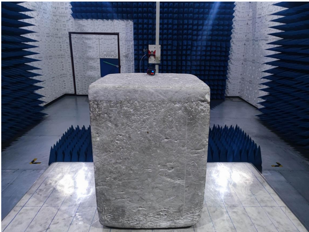
RADIATED EMISSION TEST SETUP ABOVE 1G
