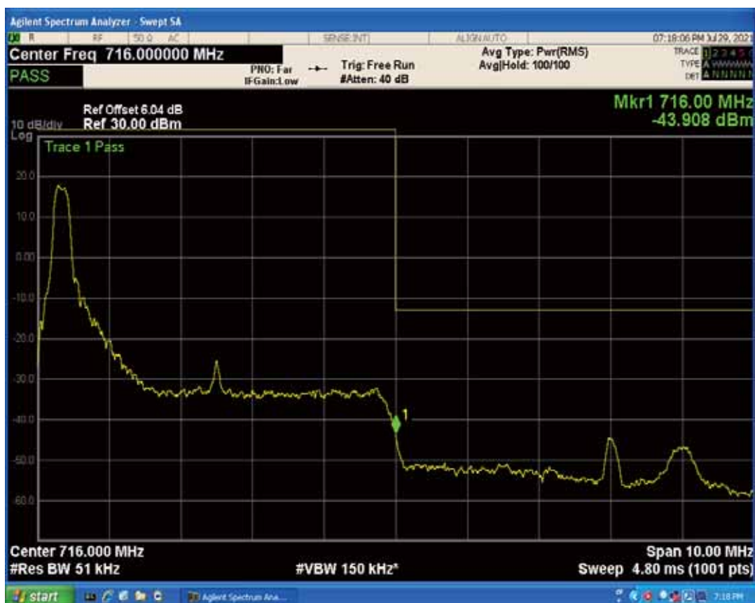
Band17 QAM16 BW=5MHz Channel=23825 RB Size=25 Position=#0
