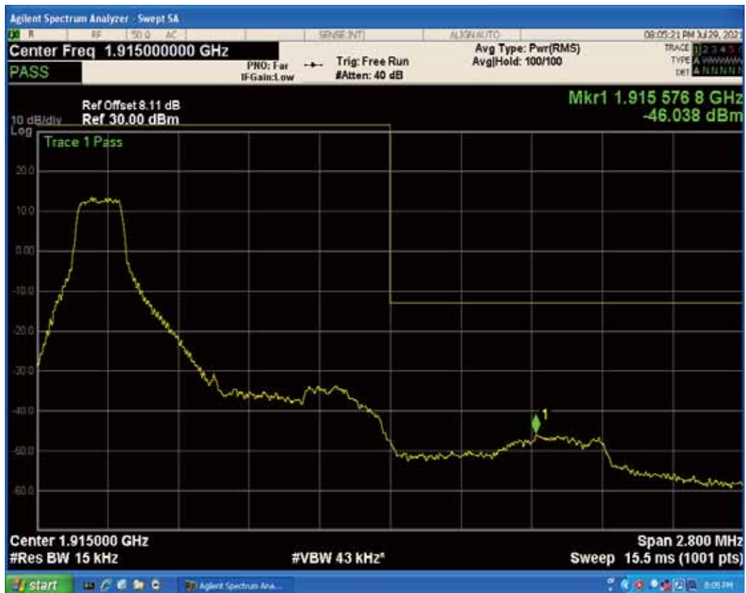
Band25 QPSK BW=1.4MHz Channel=26683 RB Size=1 Position=#Max
