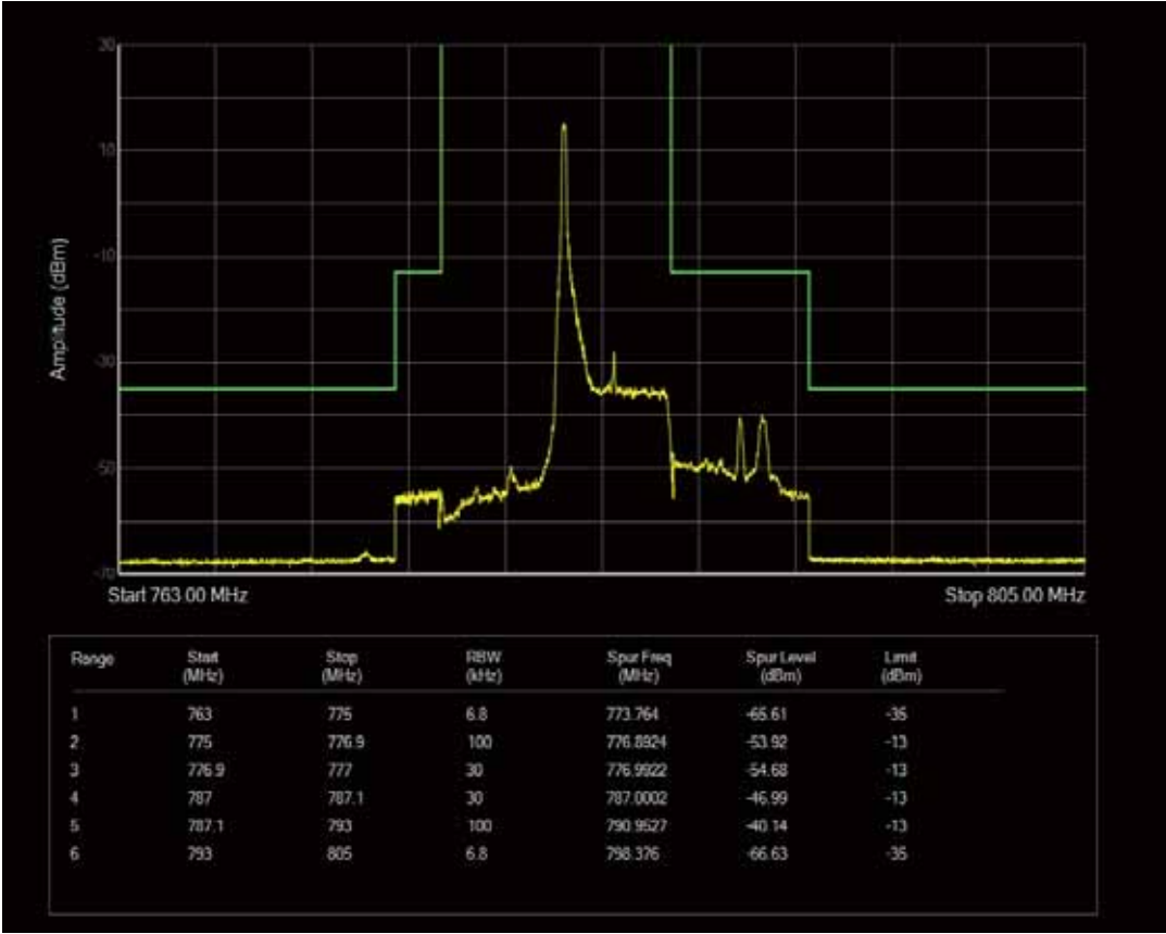
Band13 QAM16 BW=5MHz Channel=23255 RB Size=1 Position=#Max
