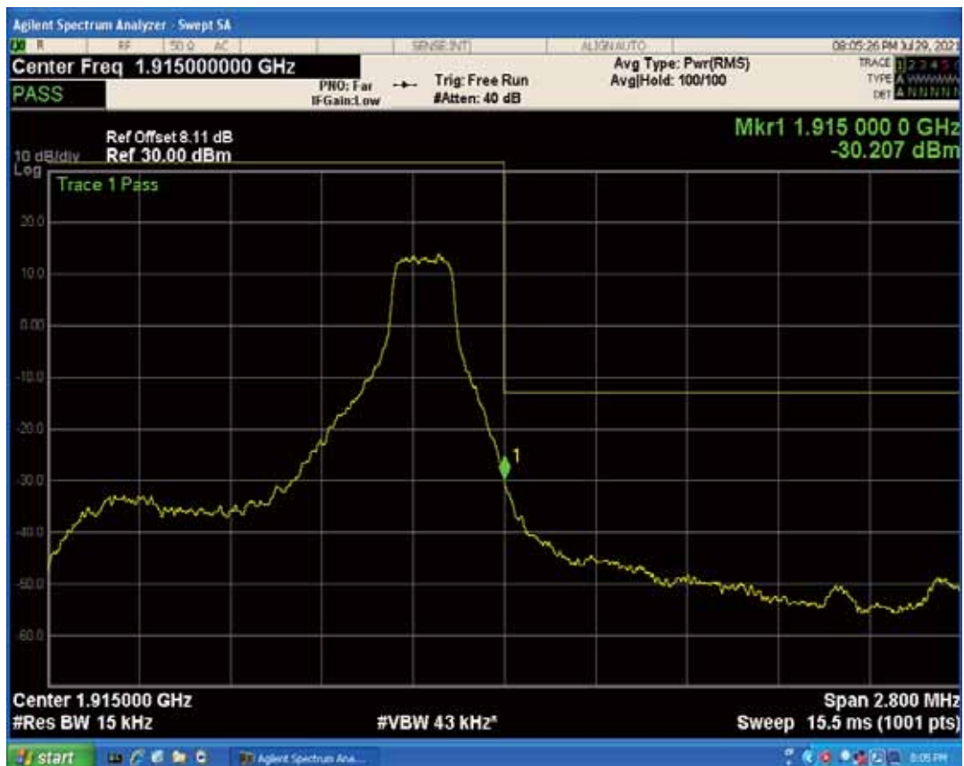
Band25 QPSK BW=1.4MHz Channel=26683 RB Size=6 Position=#0
