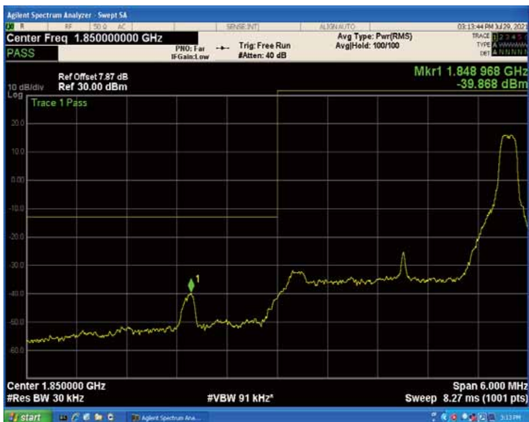
Band2 QPSK BW=3MHz Channel=18615 RB Size=1 Position=#0
