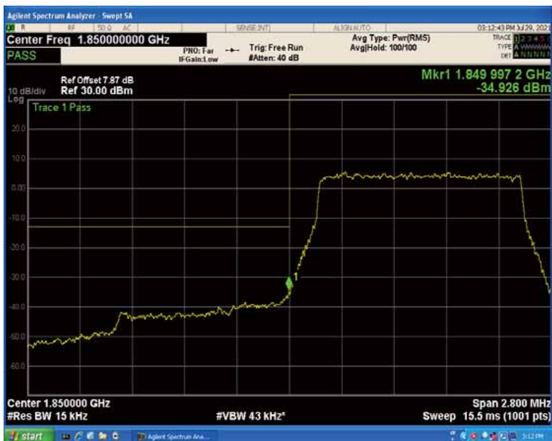
Band2 QAM16 BW=1.4MHz Channel=18607 RB Size=1 Position=#0
