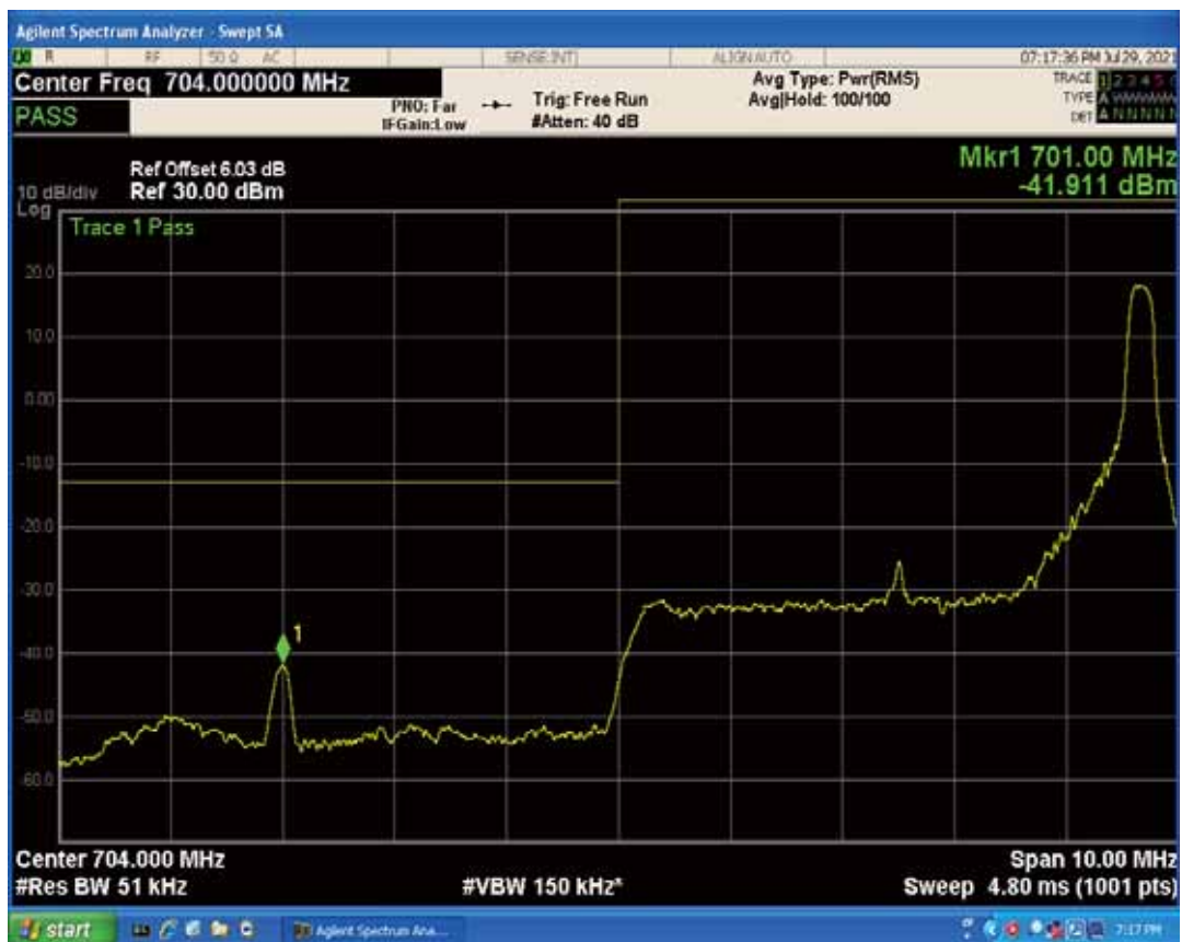
Band17 QPSK BW=5MHz Channel=23755 RB Size=1 Position=#0
