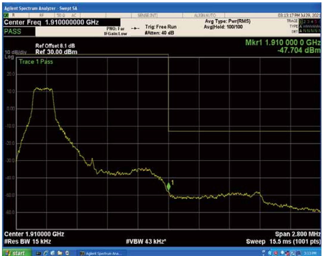
Band2 QAM16 BW=1.4MHz Channel=19193 RB Size=1 Position=#Max
