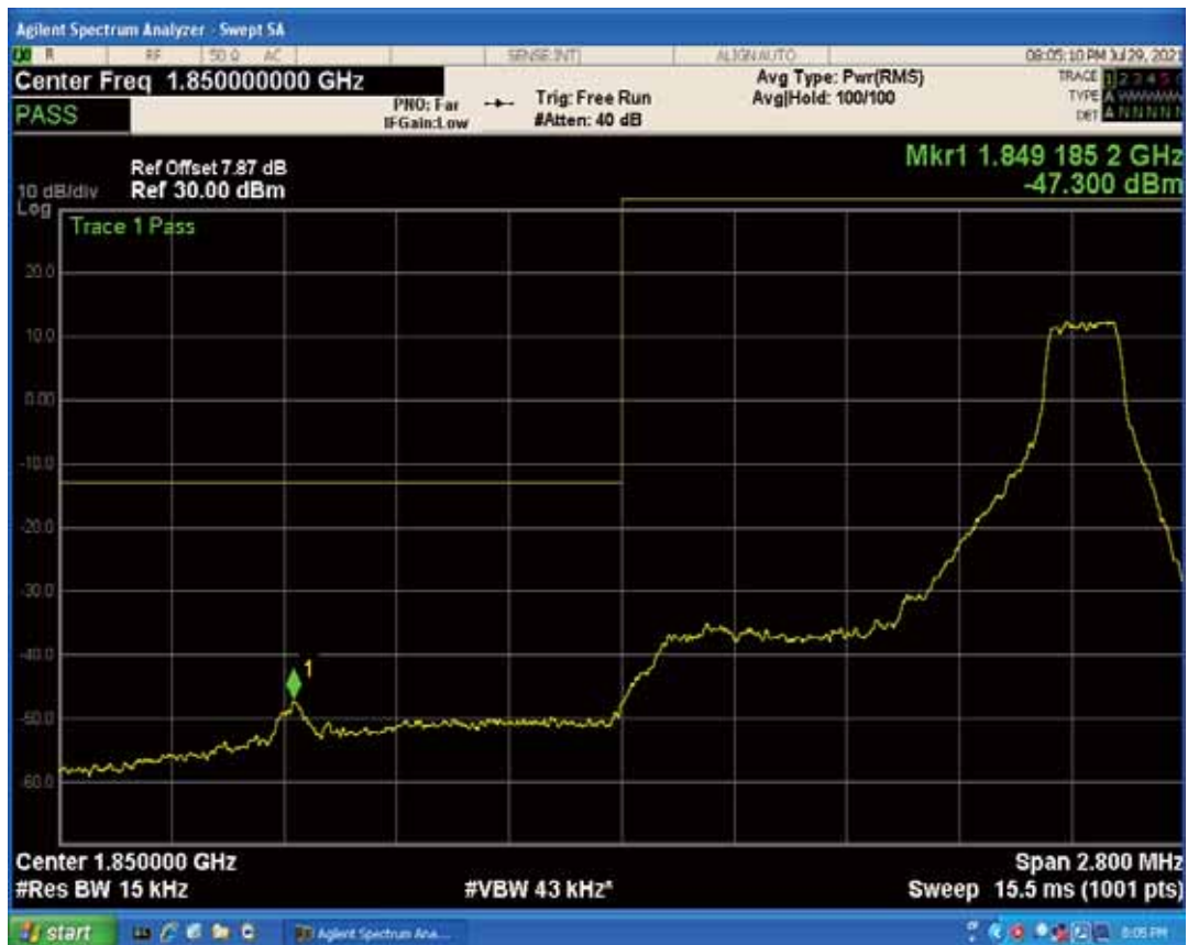
Band25 QAM16 BW=1.4MHz Channel=26047 RB Size=6 Position=#0
