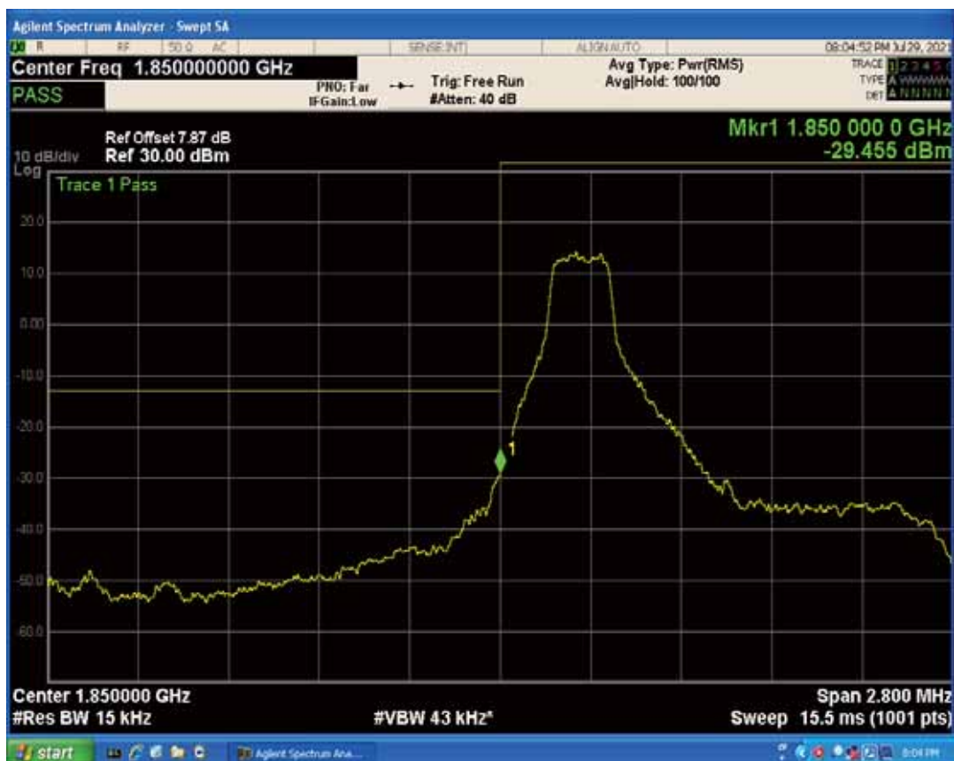
Band25 QPSK BW=1.4MHz Channel=26047 RB Size=6 Position=#0
