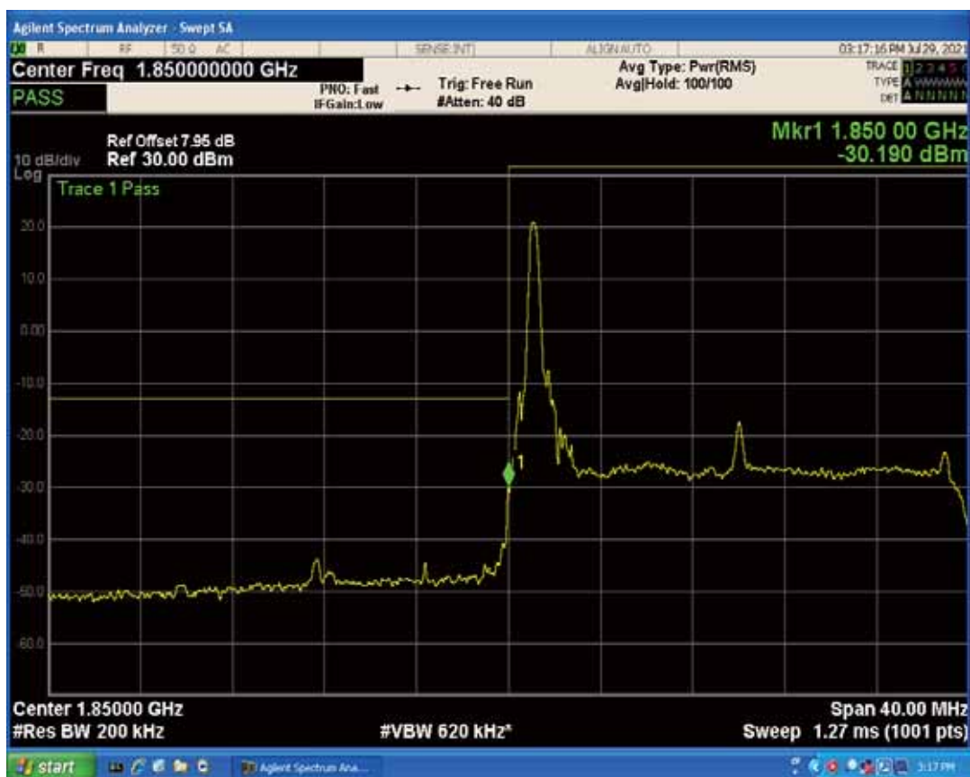
Band2 QPSK BW=20MHz Channel=19100 RB Size=1 Position=#0
