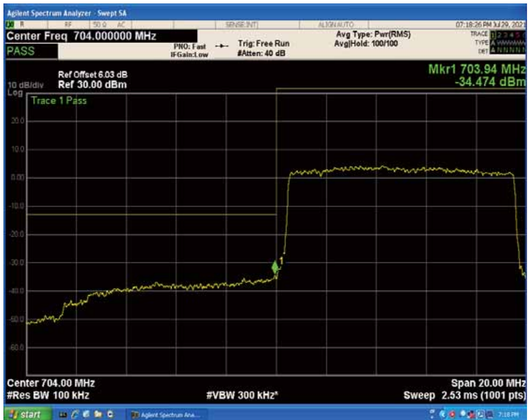
Band17 QAM16 BW=10MHz Channel=23780 RB Size=1 Position=#0
