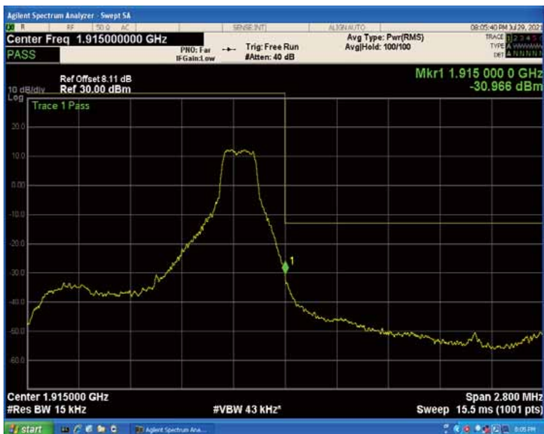
Band25 QPSK BW=3MHz Channel=26055 RB Size=1 Position=#0
