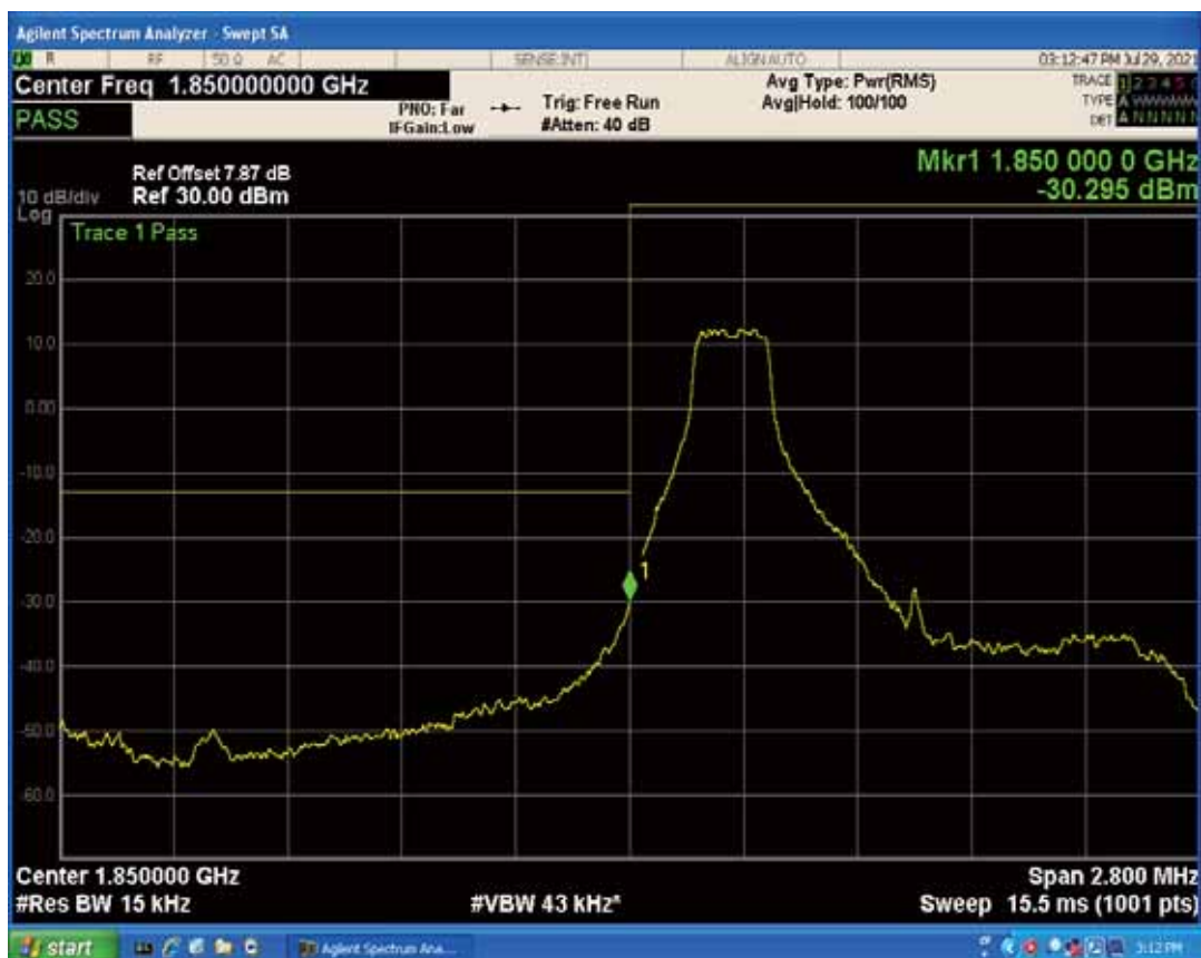
Band2 QAM16 BW=1.4MHz Channel=18607 RB Size=1 Position=#Max
