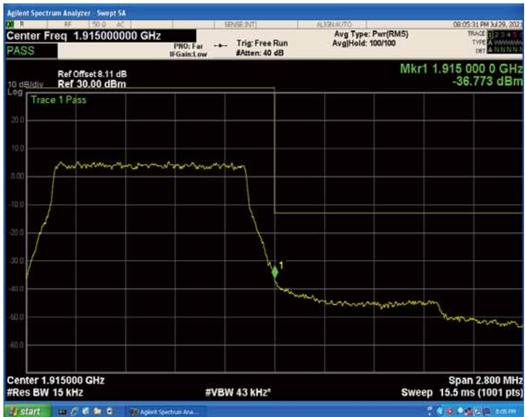
Band25 QAM16 BW=1.4MHz Channel=26683 RB Size=1 Position=#0
