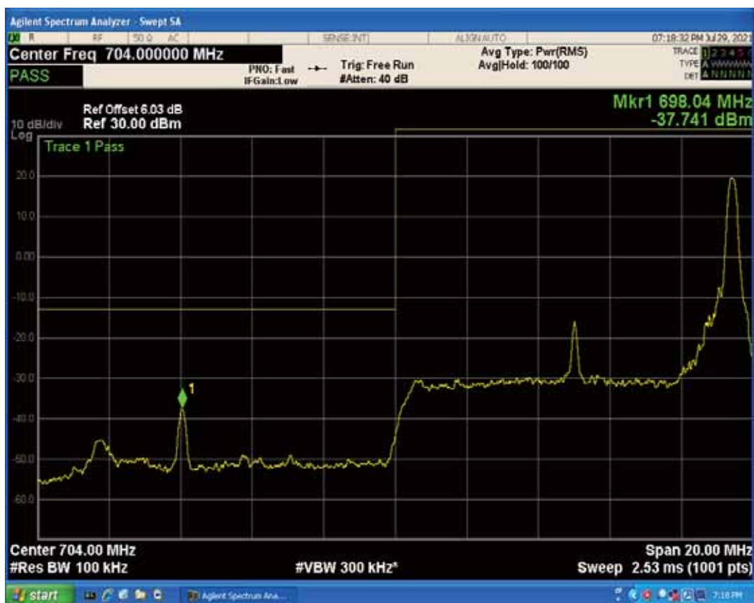
Band17 QAM16 BW=10MHz Channel=23780 RB Size=50 Position=#0
