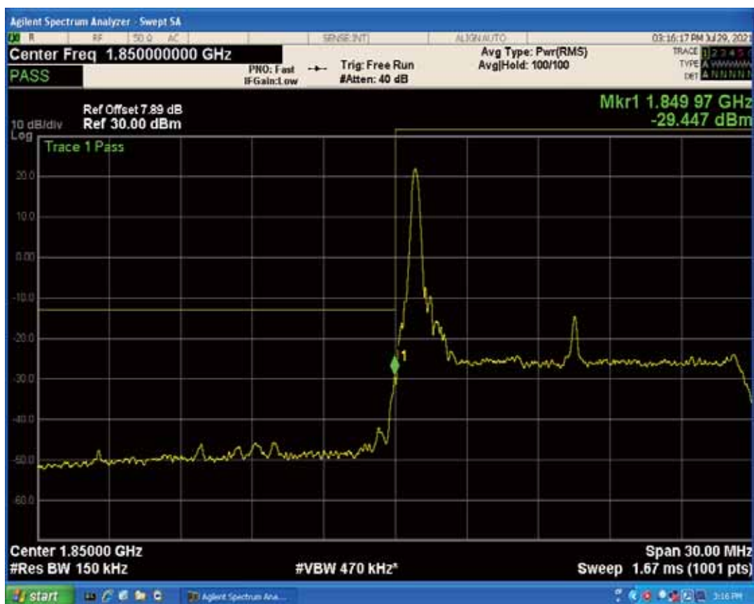
Band2 QPSK BW=15MHz Channel=18675 RB Size=1 Position=#Max
