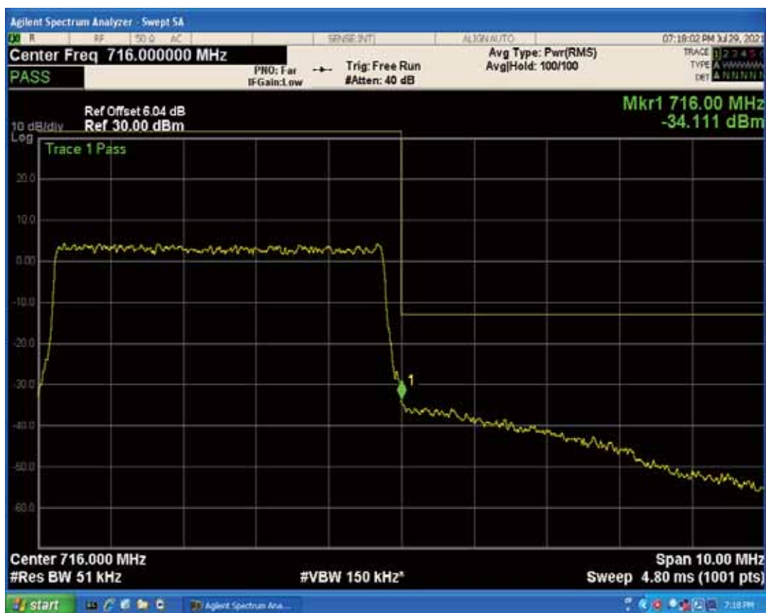
Band17 QAM16 BW=5MHz Channel=23825 RB Size=1 Position=#Max
