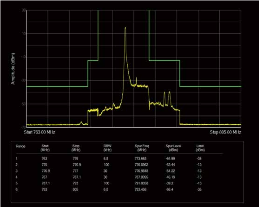
Band13 QPSK BW=5MHz Channel=23255 RB Size=1 Position=#Max
