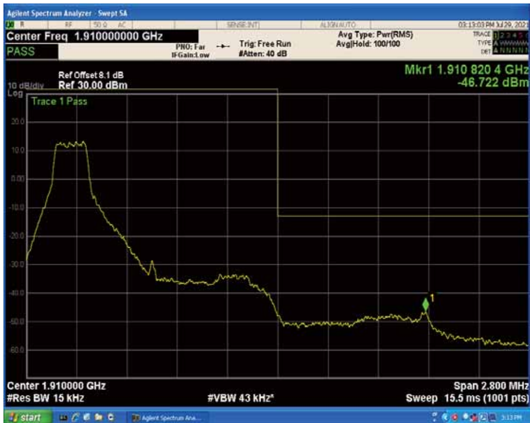
Band2 QPSK BW=1.4MHz Channel=19193 RB Size=1 Position=#Max
