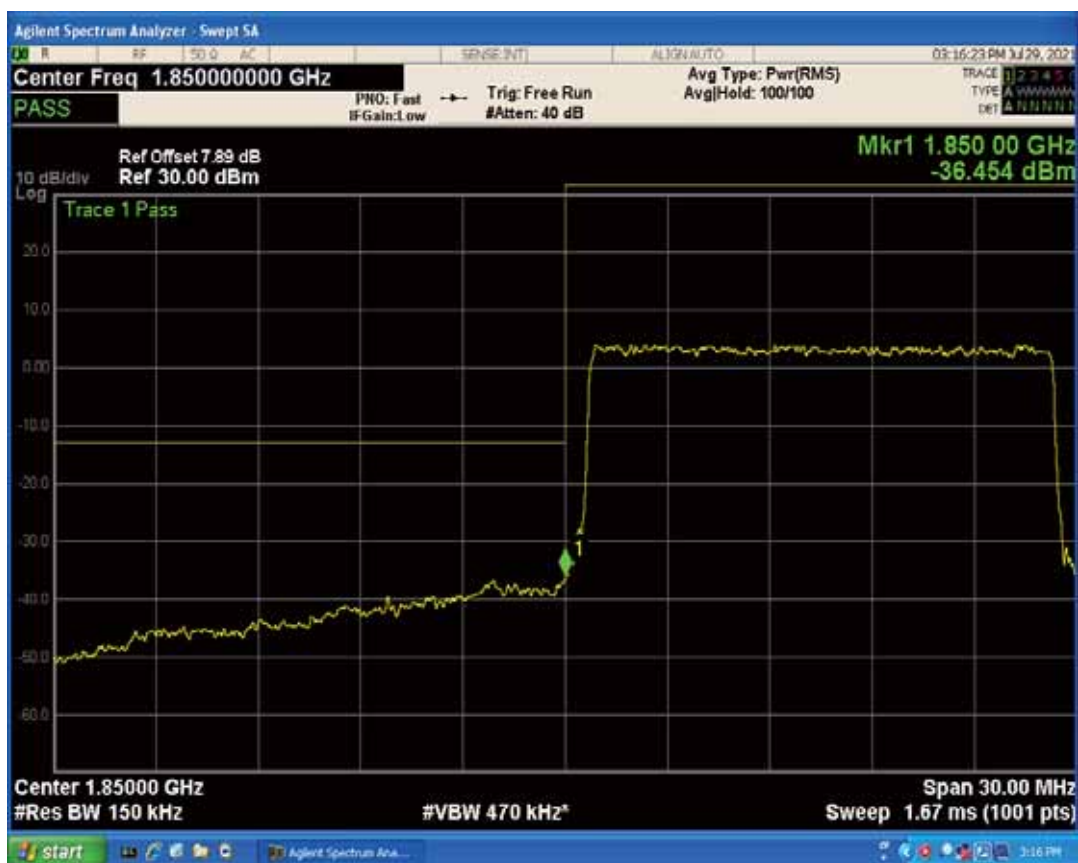
Band2 QAM16 BW=15MHz Channel=18675 RB Size=1 Position=#Max
