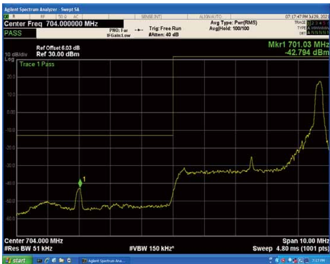
Band17 QAM16 BW=5MHz Channel=23755 RB Size=25 Position=#0
