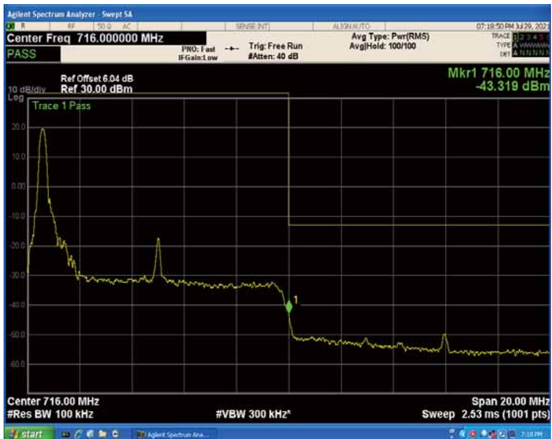
Band17 QAM16 BW=10MHz Channel=23800 RB Size=1 Position=#Max
