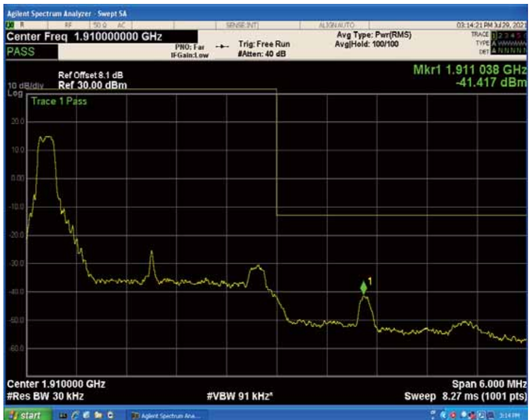
Band2 QAM16 BW=3MHz Channel=19185 RB Size=1 Position=#Max
