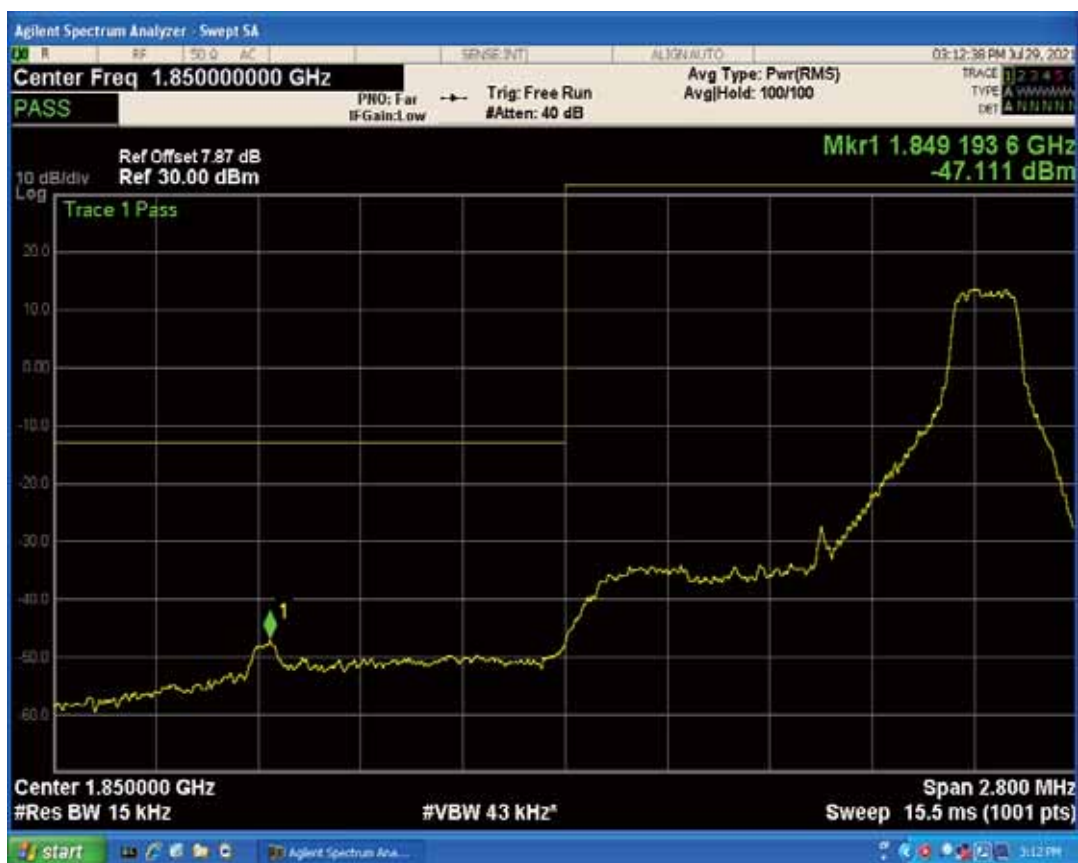
Band2 QPSK BW=1.4MHz Channel=18607 RB Size=1 Position=#0
