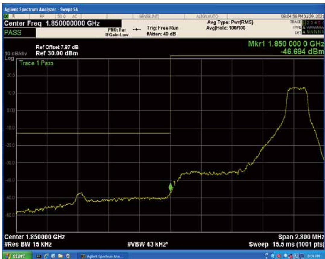
Band25 QPSK BW=1.4MHz Channel=26047 RB Size=1 Position=#0
