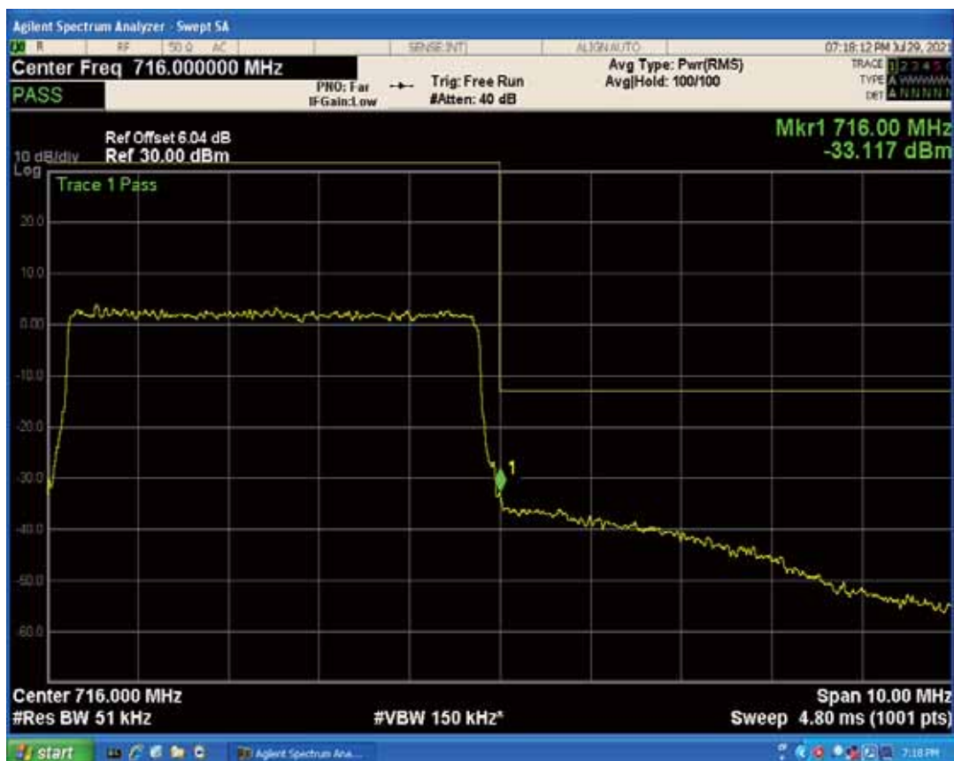
Band17 QPSK BW=10MHz Channel=23780 RB Size=1 Position=#Max
