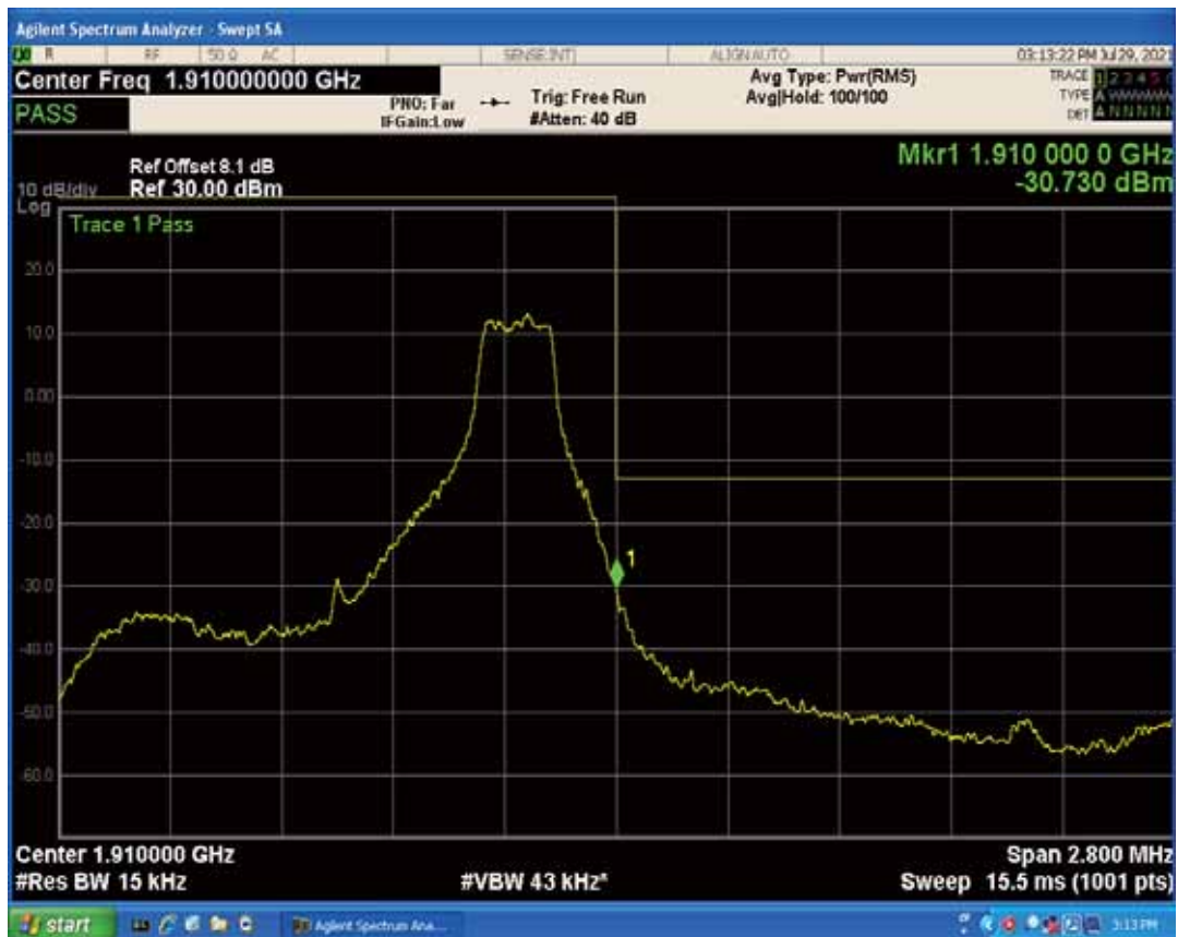
Band2 QAM16 BW=1.4MHz Channel=19193 RB Size=6 Position=#0
