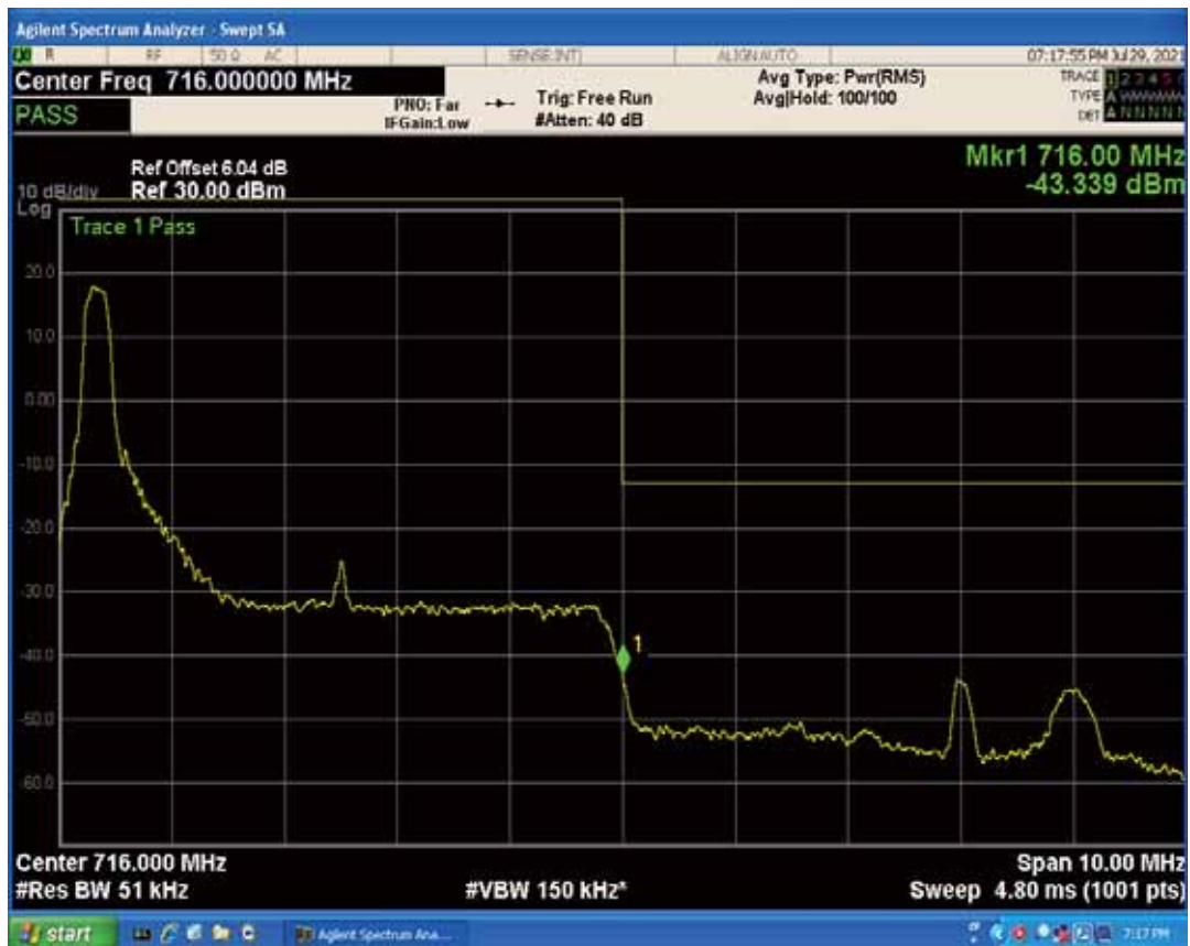
Band17 QPSK BW=5MHz Channel=23825 RB Size=1 Position=#Max
