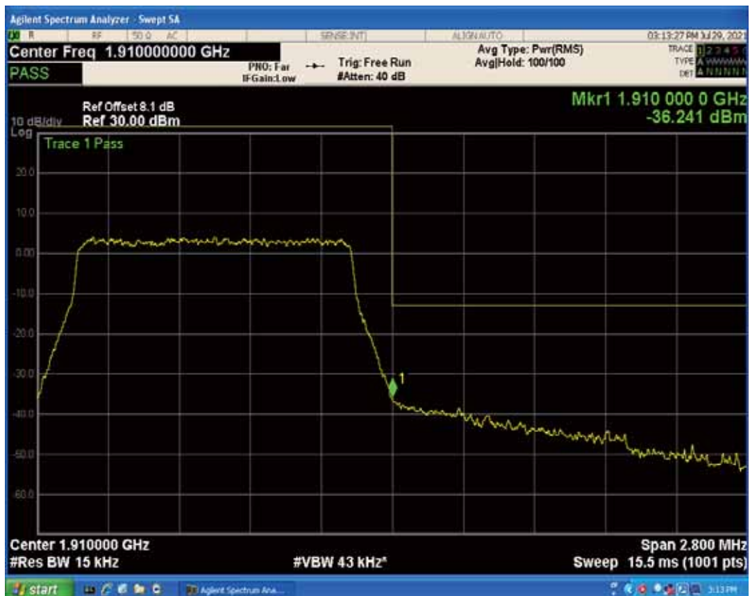
Band2 QPSK BW=3MHz Channel=18615 RB Size=1 Position=#Max
