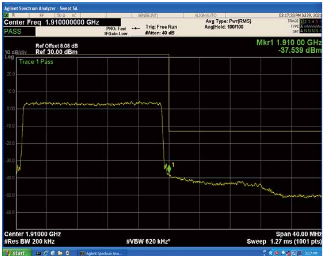
Band2 QAM16 BW=20MHz Channel=19100 RB Size=1 Position=#Max
