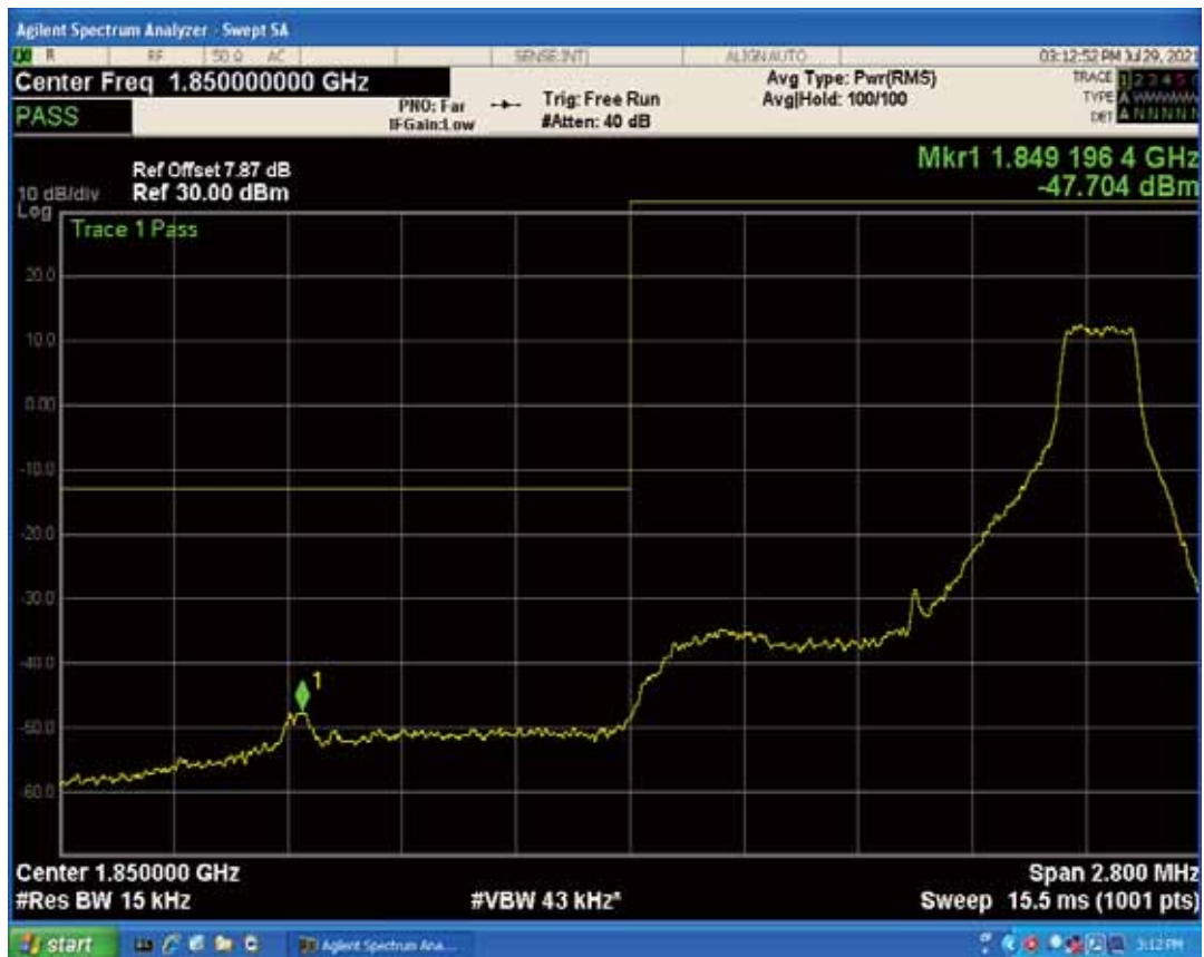
Band2 QAM16 BW=1.4MHz Channel=18607 RB Size=6 Position=#0
