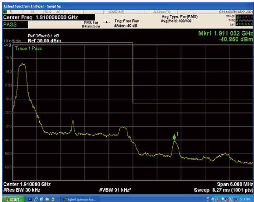
Band2 QPSK BW=3MHz Channel=19185 RB Size=1 Position=#Max
