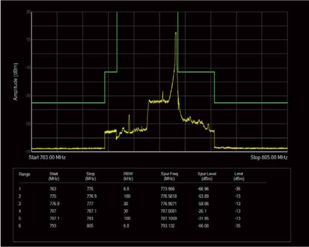
Band13 QPSK BW=5MHz Channel=23255 RB Size=25 Position=#0
