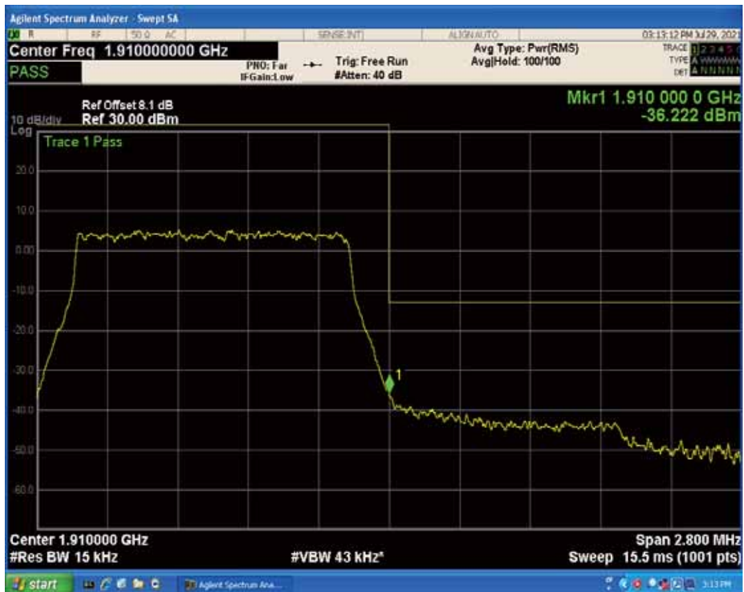
Band2 QAM16 BW=1.4MHz Channel=19193 RB Size=1 Position=#0
