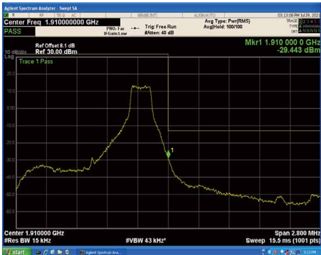
Band2 QPSK BW=1.4MHz Channel=19193 RB Size=6 Position=#0
