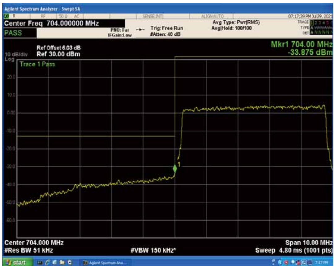
Band17 QAM16 BW=5MHz Channel=23755 RB Size=1 Position=#0
