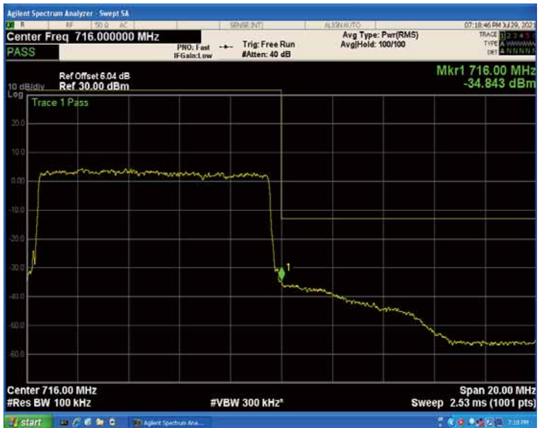
Band17 QAM16 BW=10MHz Channel=23800 RB Size=1 Position=#0
