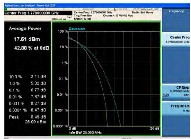
Band66 / 20MHz / High CH / 64QAM
