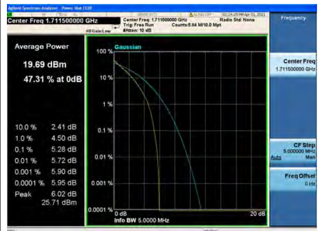
Band66 / 3MHz / Low CH / 64QAM
