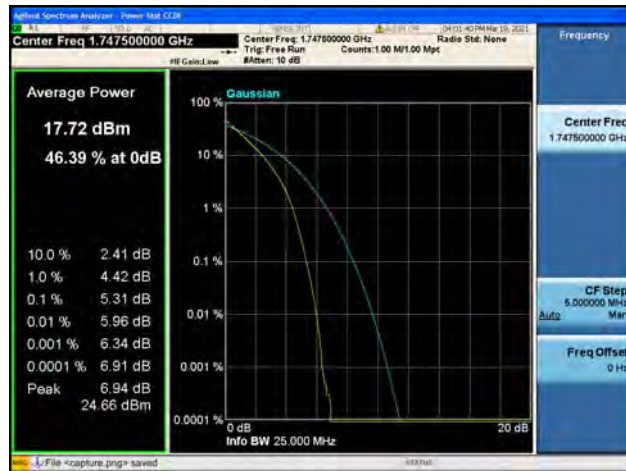
Band4 / 15MHz / High CH / 64QAM
