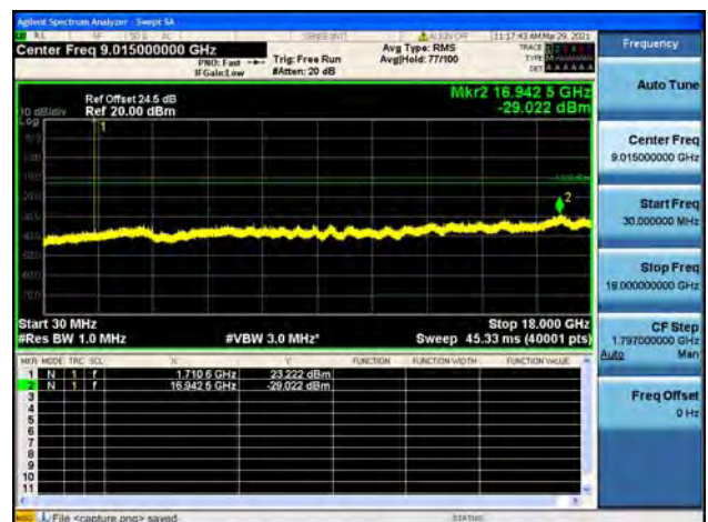
Band4 / 3MHz / Low CH / 64QAM
