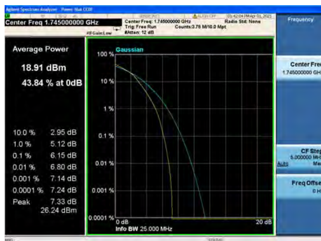
Band66 / 15MHz / Mid CH / 16QAM
