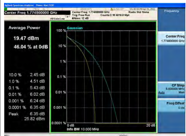
Band66 / 10MHz / High CH / 64QAM
