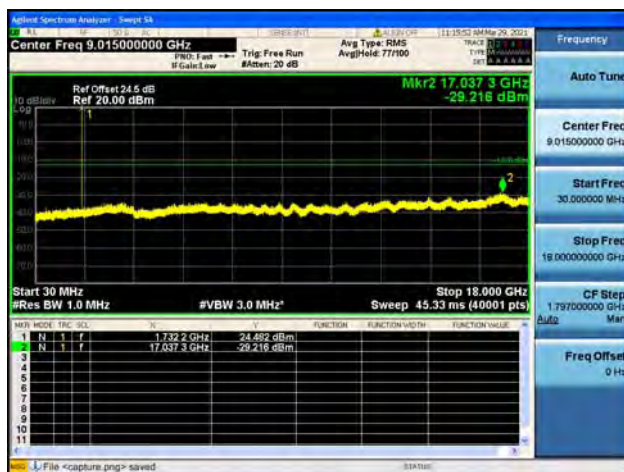
Band4 / 1.4MHz / Mid CH / 16QAM
