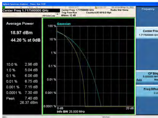
Band66 / 15MHz / Mid CH / 16QAM
