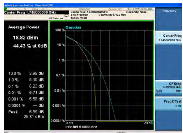
Band66 / 1.4MHz / Mid CH / 64QAM
