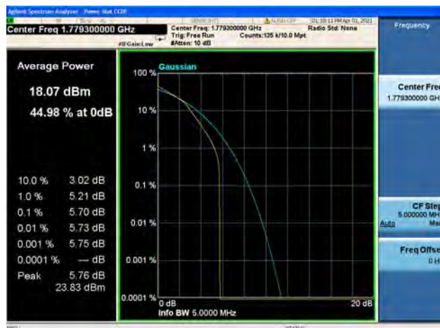
Band66 / 3MHz / Low CH / 16QAM
