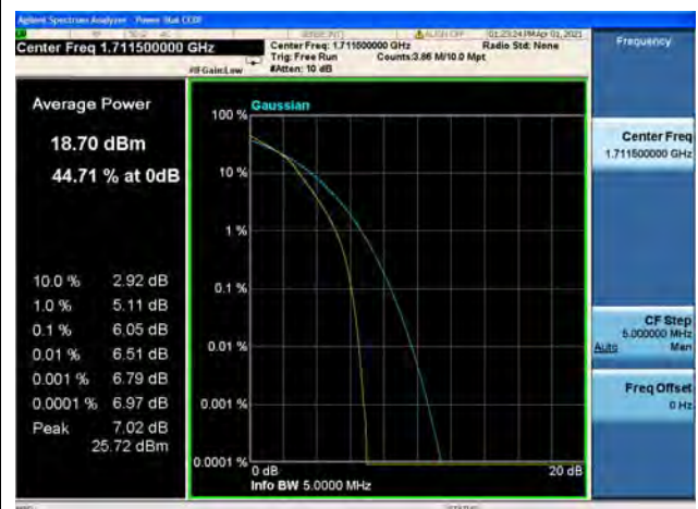
Band66 / 3MHz / Low CH / 64QAM
