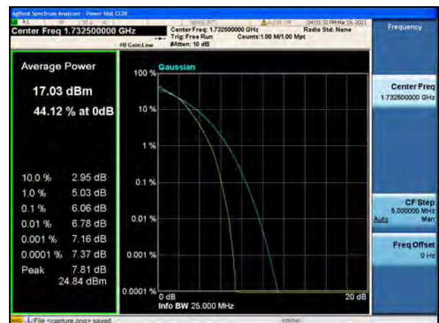
Band4 / 15MHz / Mid CH / 64QAM
