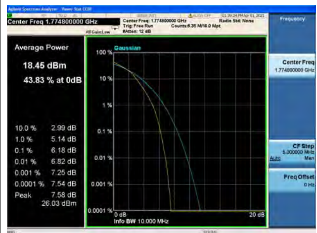
Band66 / 10MHz / High CH / 64QAM
