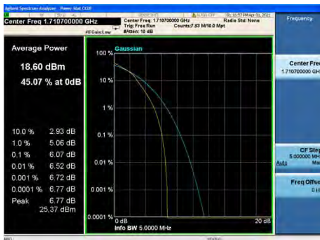
Band66 / 1.4MHz / Mid CH / 16QAM
