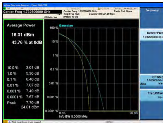
Band4 / 1.4MHz / Mid CH / 16QAM
