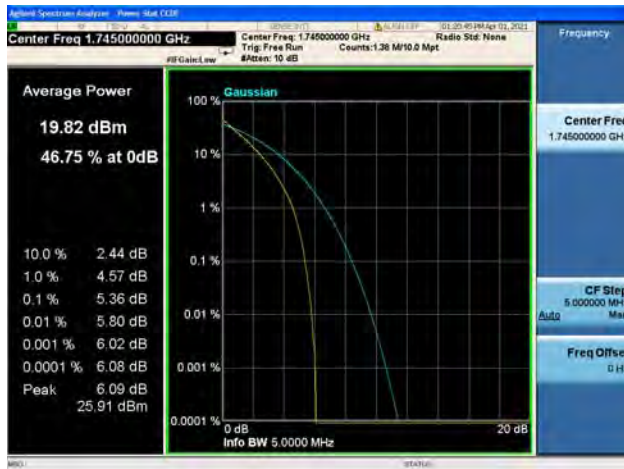
Band66 / 3MHz / Mid CH / 64QAM
