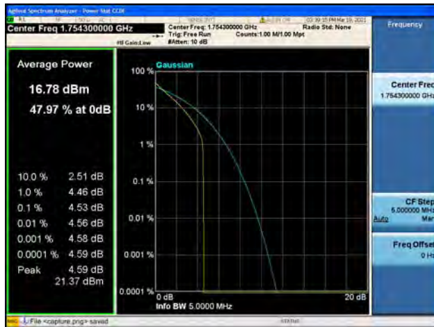
Band4 / 1.4MHz / High CH / 64QAM
