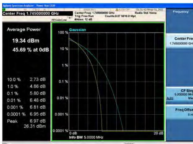
Band66 / 5MHz / Mid CH / 16QAM
