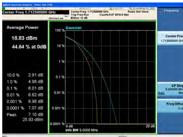
Band66 / 5MHz / Mid CH / 16QAM
