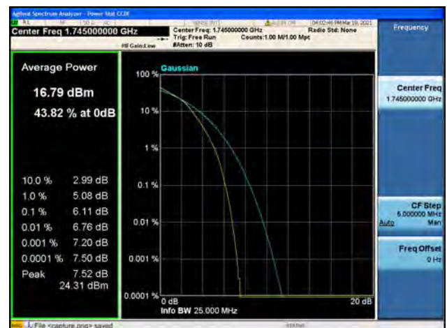
Band4 / 20MHz / High CH / 64QAM
