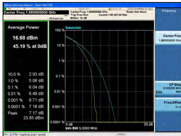
Band2 / 3MHz / High CH / 16QAM
