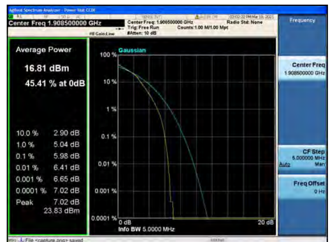
Band2 / 3MHz / High CH / 64QAM
