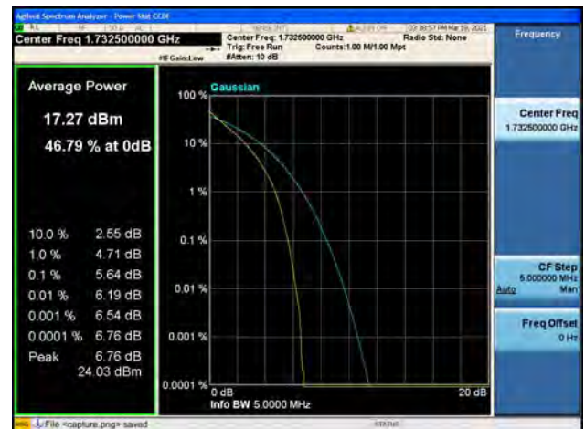
Band4 / 1.4MHz / Mid CH / 64QAM
