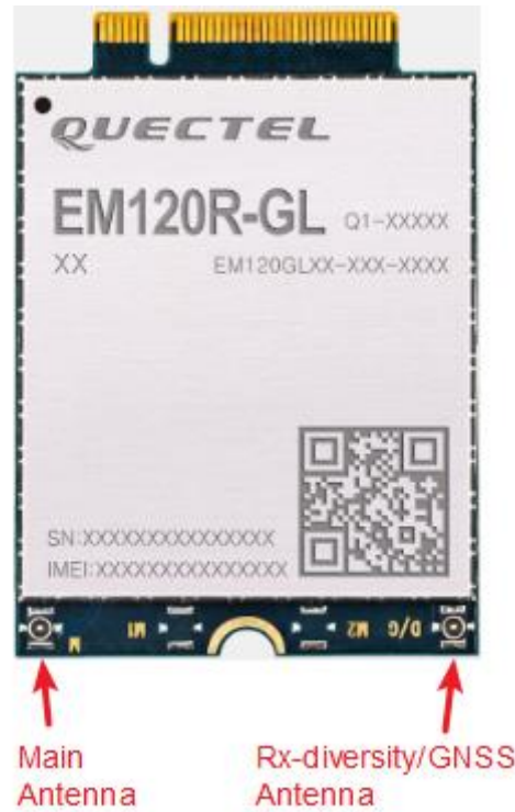
Figure 33: Antenna Connectors on the EM120R-GL Module
