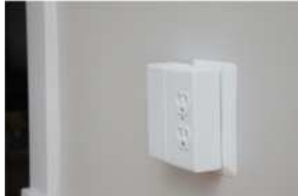
Figure 10: Side view of Location Beacon AC Power (right) with Access Point attached (left)
