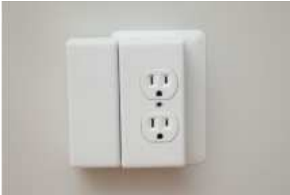
Figure 5: Location Beacon AC Power with external power cable inserted.
