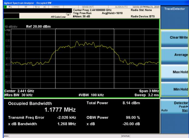
20dB Bandwidth plot on channel 78 (1Mbps)
