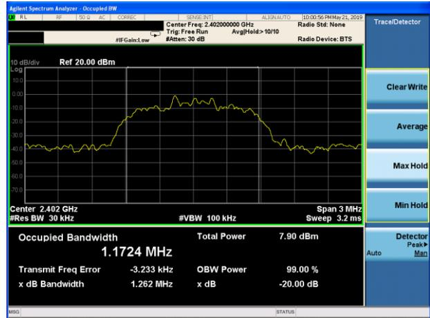
20dB Bandwidth plot on channel 39 (1Mbps)
