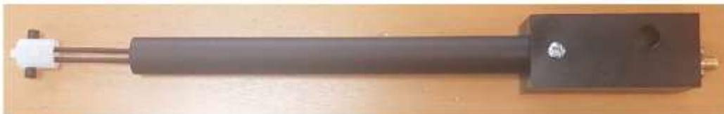
**Figure 1 – MVG COMOSAR Validation Dipole**
