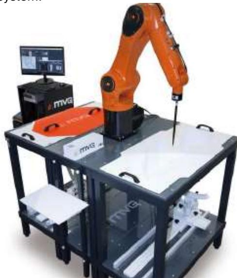
The EUT under test operating at the maximum power level is placed in the phone holder, under the phantom, which is filled with head simulating liquid. The E-Field probe measures the electric field inside the phantom. The OpenSAR software computes the results to give a SAR value in a 1g or 10g mass.
