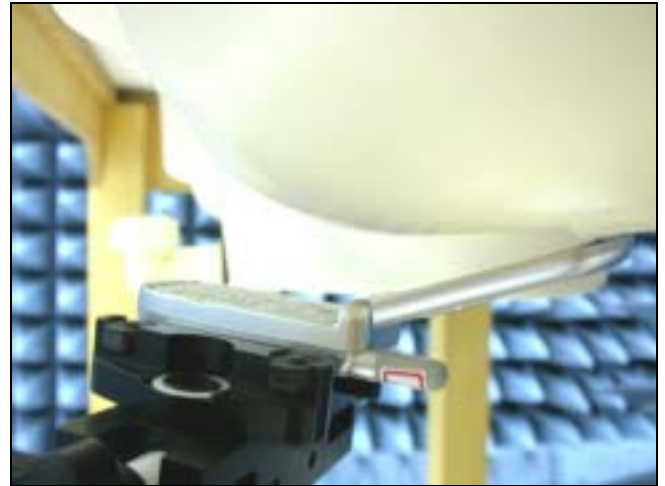
Figure 15. Left Head SAR Test Setup (Tilted)
