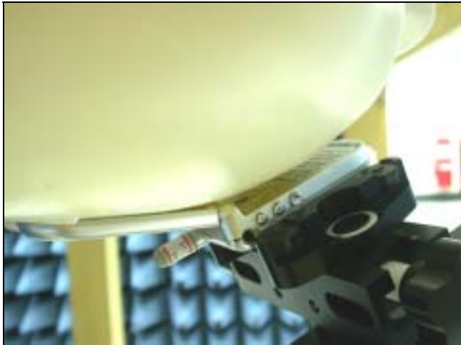
Figure 16. Right Head SAR Test Setup (Cheek)
