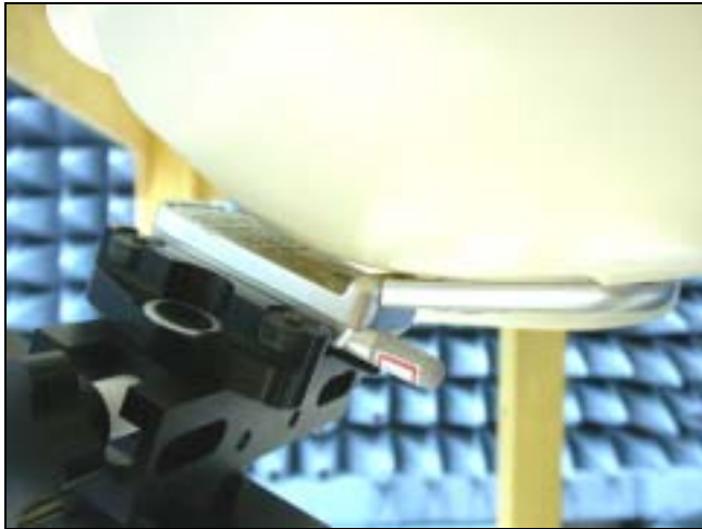
Figure 14. Left Head SAR Test Setup (Cheek)
