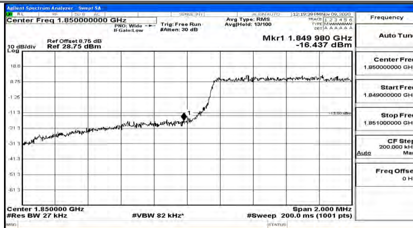
Band Edge Test Graph(s) (Channel Bandwidth: 1.4 MHz)_LCH_QPSK
