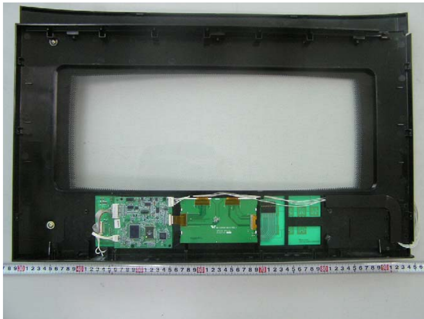
EUT- Control Unit View
