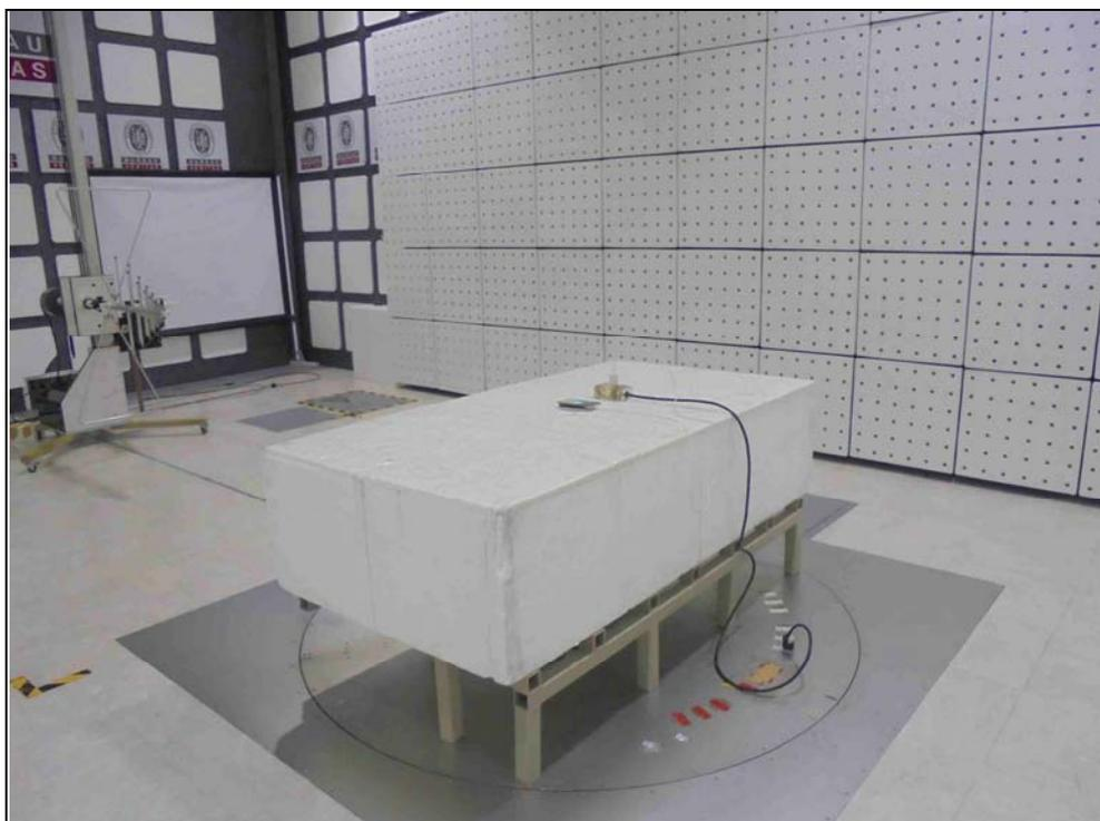
RADIATED EMISSION TEST (Mode E)
