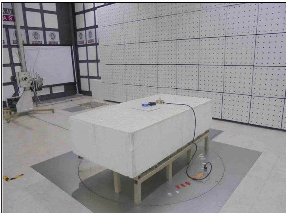
RADIATED EMISSION TEST (Mode C)
