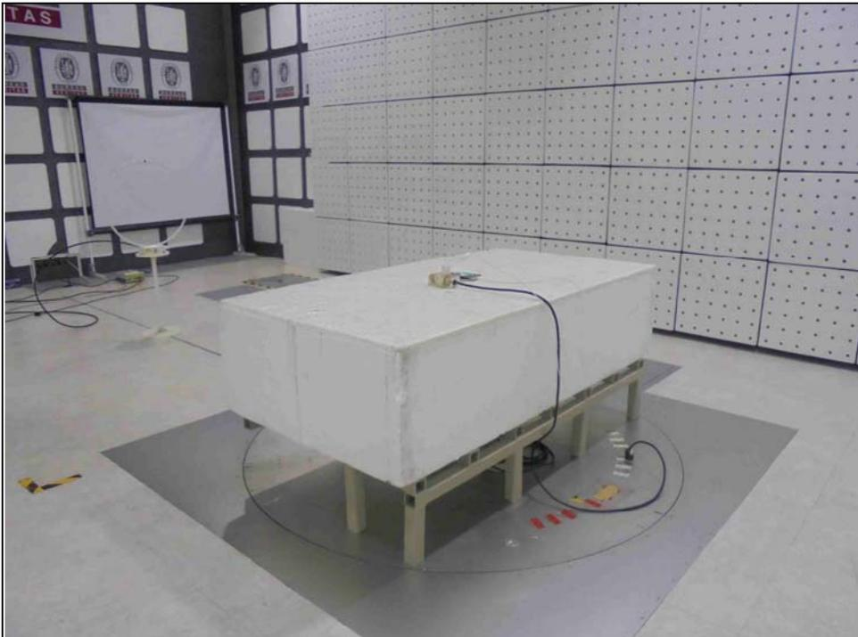
RADIATED EMISSION TEST (Mode E)
