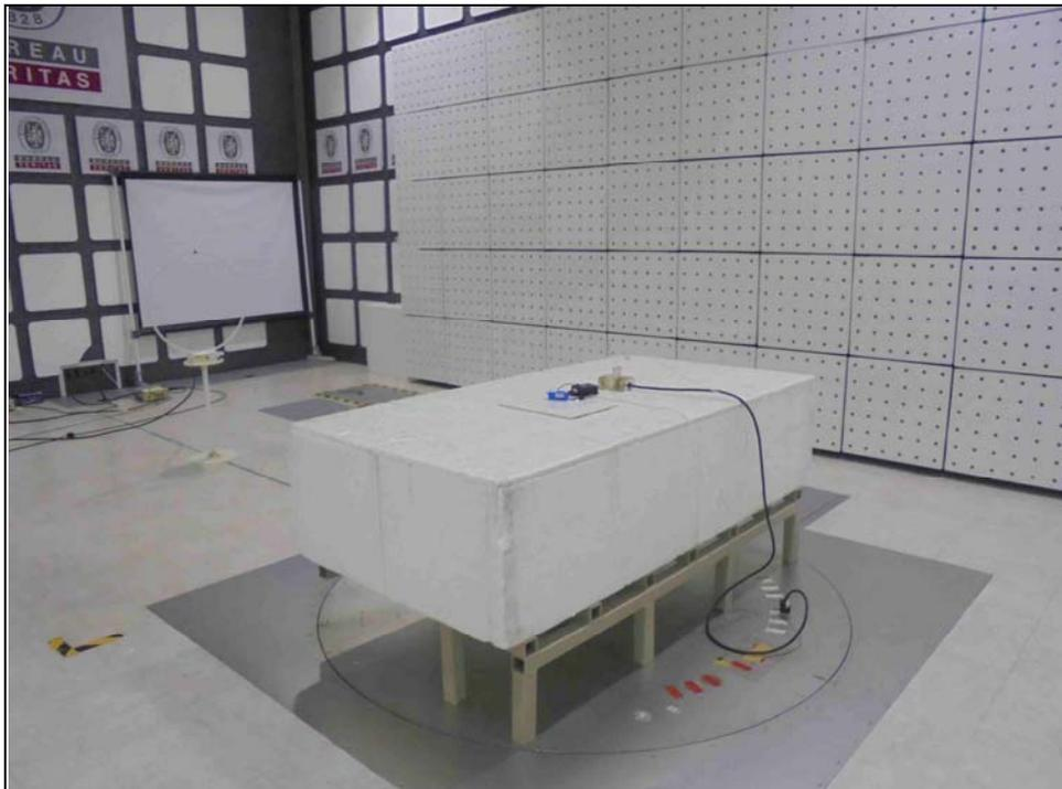
RADIATED EMISSION TEST (Mode C)
