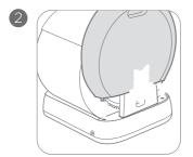
Insert the rear cover into the slot of the base.
