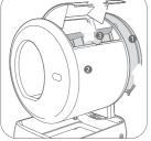
Clean up the waste bin, then unplug the litter box. Take out the rear cover first then hold to take out the drum.
