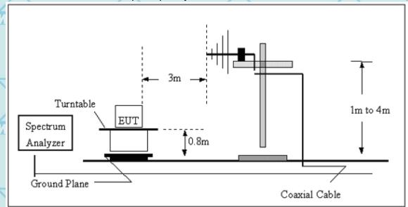
(B) Radiated Emission Test-Up Frequency Above 1GHz
