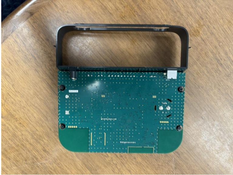
Internal mask part with PCB attached back
