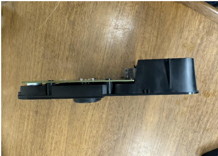
Internal mask part with PCB attached side
