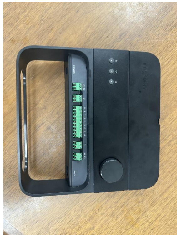
Internal mask part with PCB attached front
