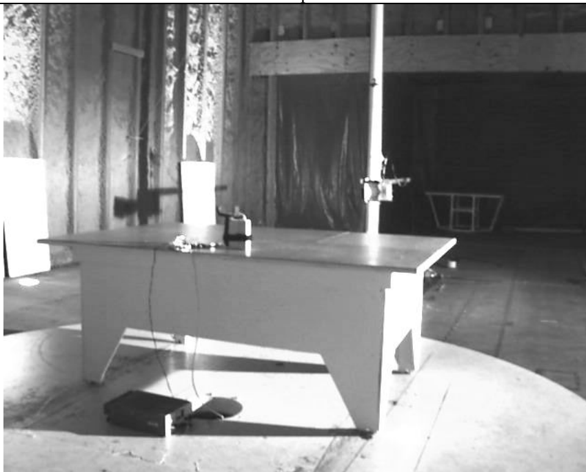
Emissions Set Up Below 1 GHz
