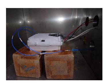
Photograph No.5 Frequency stability measurement setup
