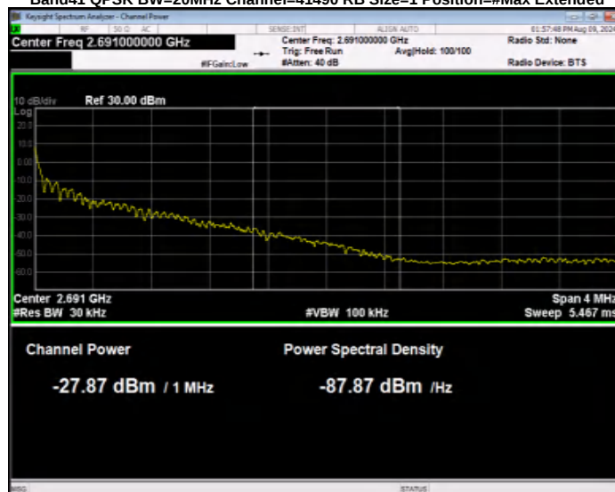
Band41 QPSK BW=20MHz Channel=41490 RB Size=1 Position=#Max Normal
