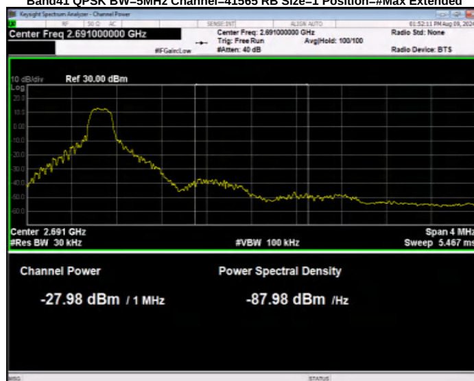
Band41 QPSK BW=5MHz Channel=41565 RB Size=1 Position=#Max Normal
