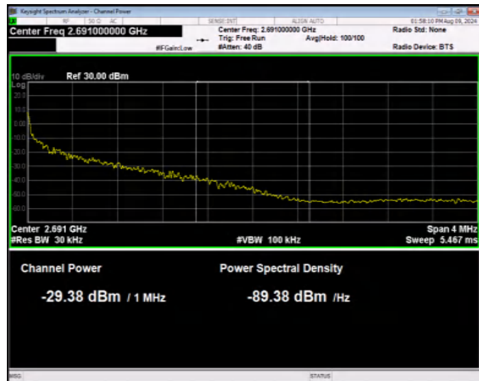
Band41 16QAM BW=20MHz Channel=41490 RB Size=1 Position=#Max Normal
