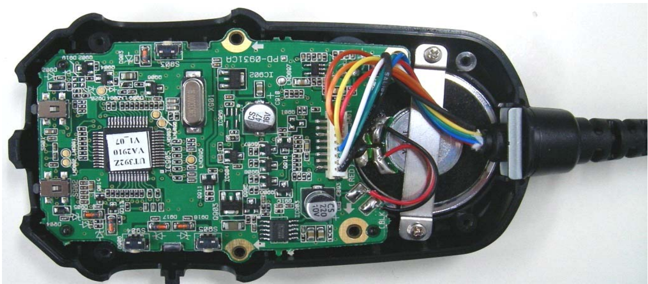
Remote MIC PCB Top View
