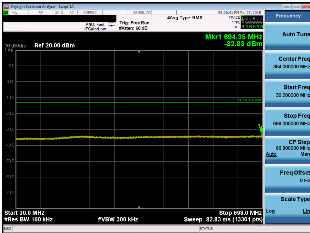
Plot 7-85. Conducted Spurious Plot (Band 12/17 - 10.0MHz QPSK - RB Size 1, RB Offset 0 - Mid Channel)
