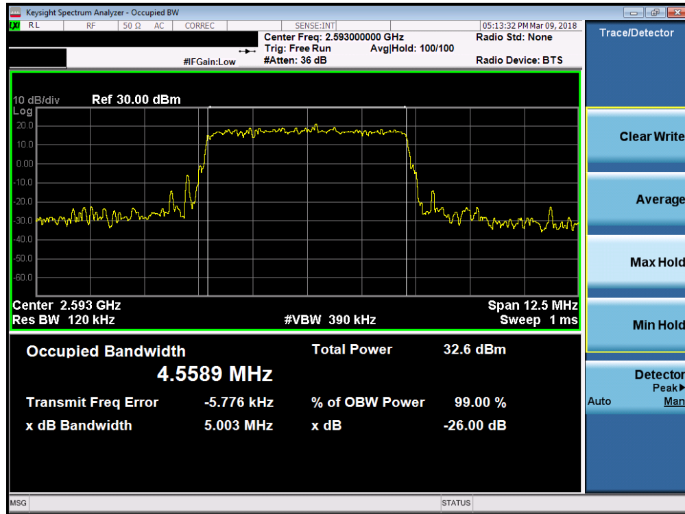
Plot 7-70. Occupied Bandwidth Plot (Band 41 - 5.0MHz QPSK - Full RB Configuration)
