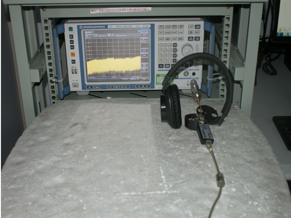
Photograph 2: Set-up for Spurious Emissions (9kHz-30MHz)
