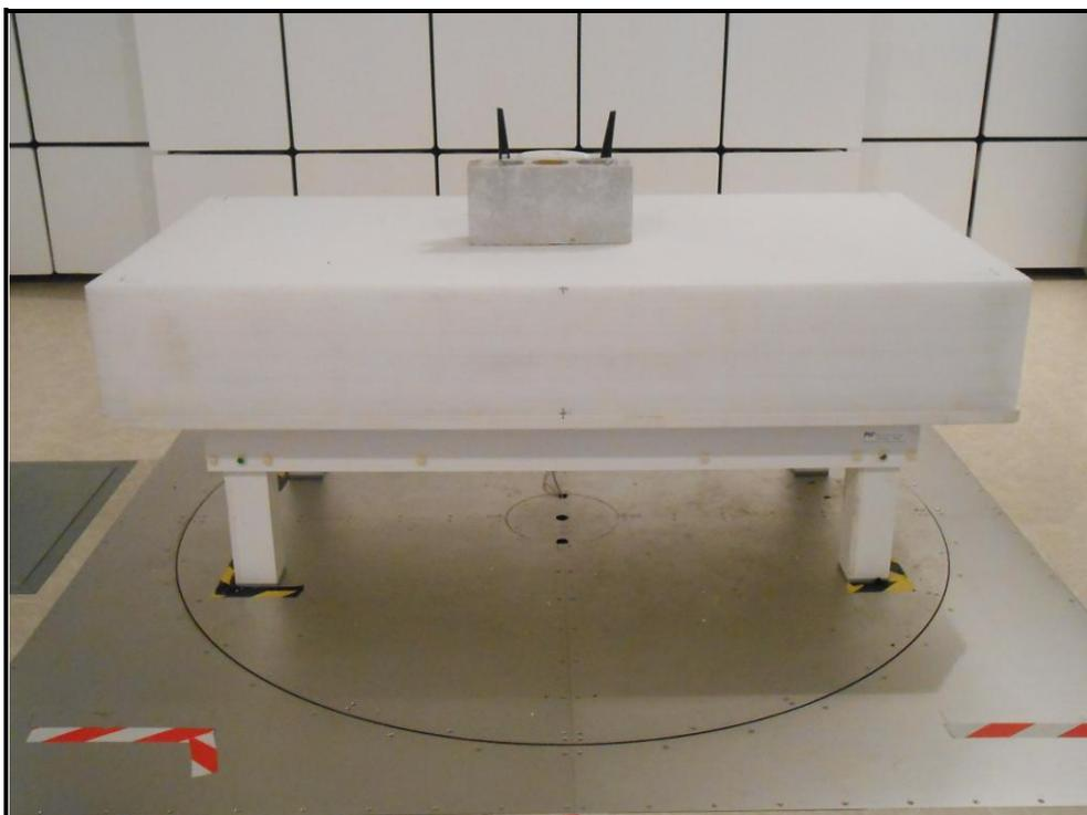
RADIATED EMISSION TEST (Above 1GHz – with internal antenna)
