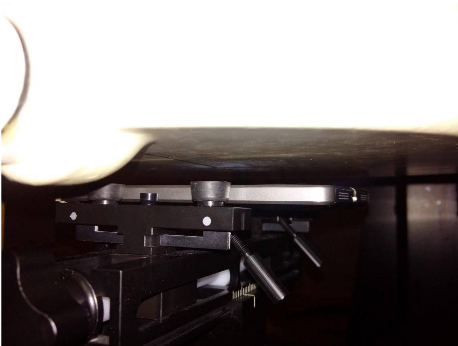
Figure E7. Hotspot configuration (No Holster, front side 10mm away)
