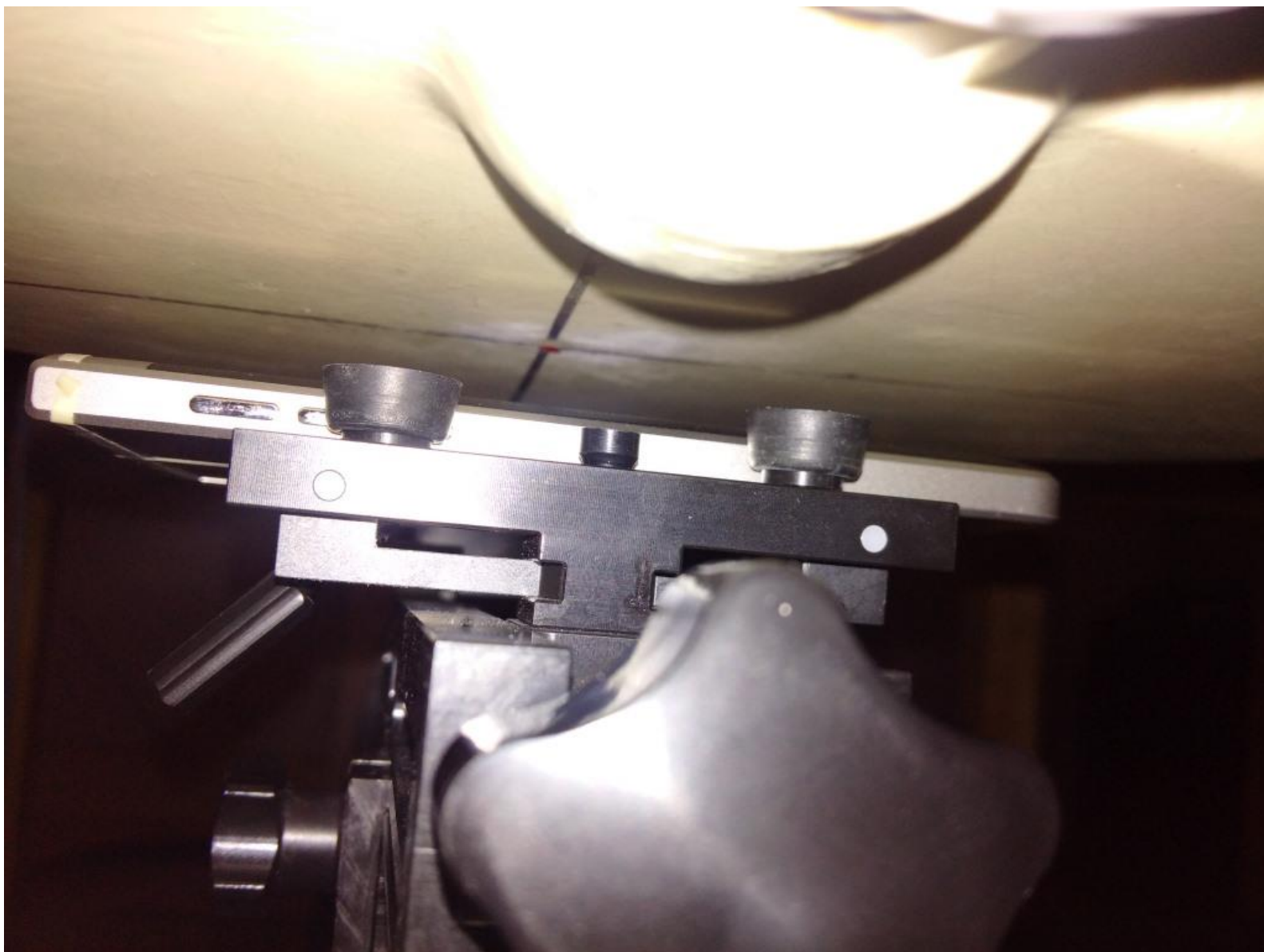
Figure E13. Body-worn configuration (No Holster, back side 15mm away)
