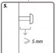
It is advisable to leave no more than 5mm between the head of the screw and the wall to minimise the inclination angle of the Soundbar.
