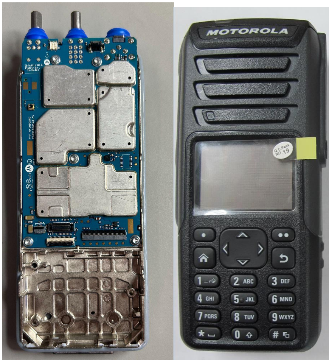
RF board with chasis and housing (front) Model 3 (VX-P949)
