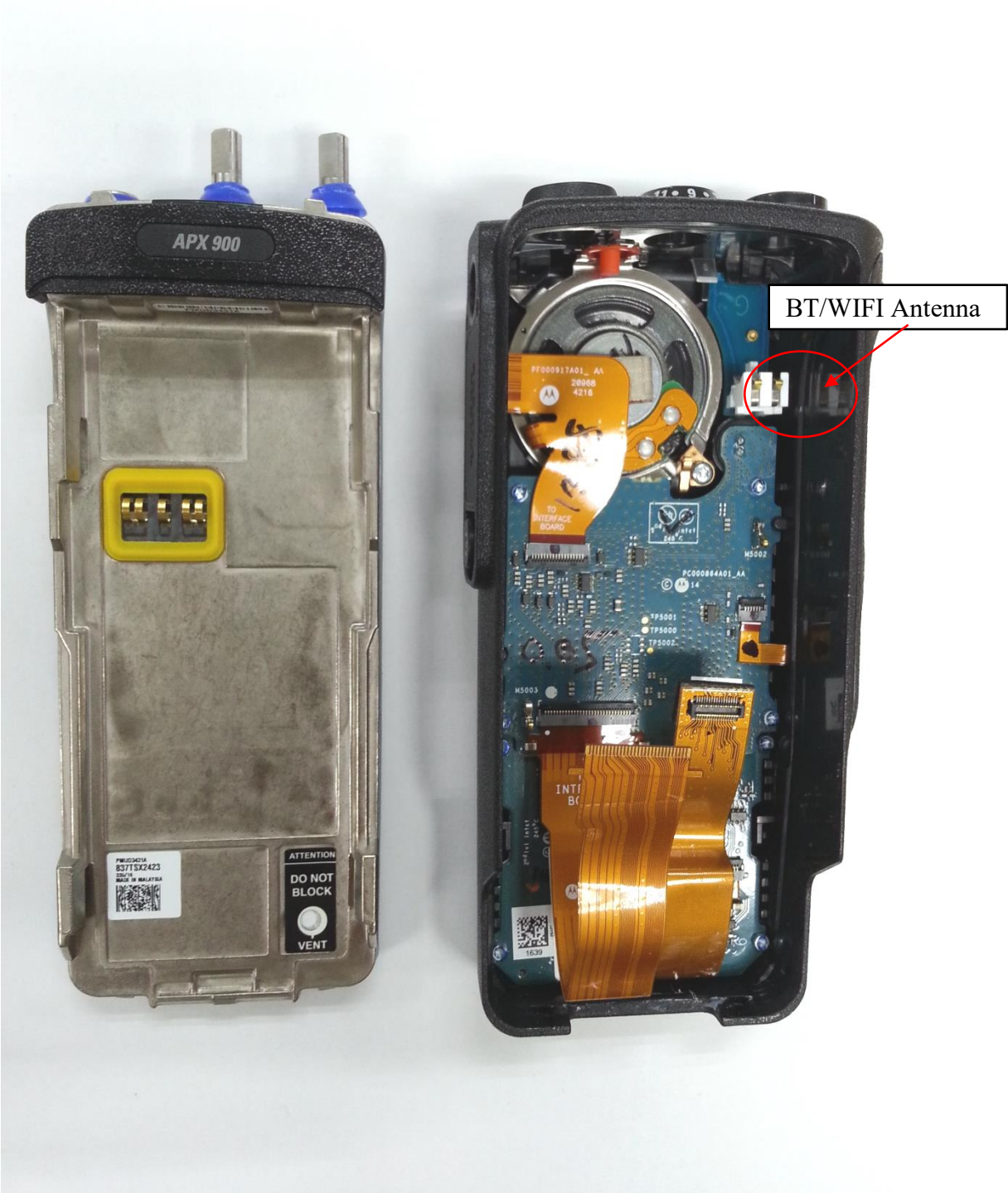
Chassis and Housing (Back), Model 2 (APX900)
