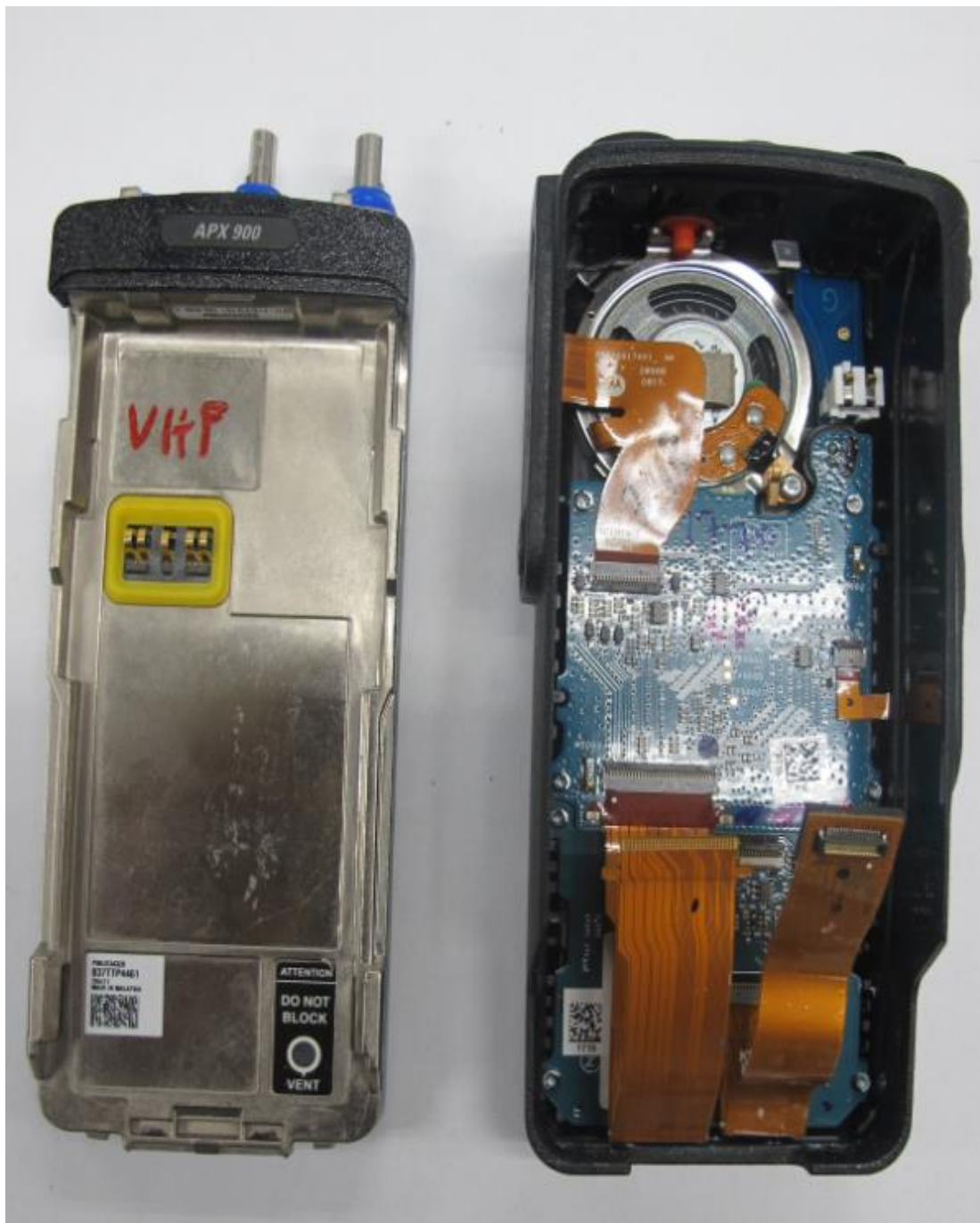
Chassis and Housing (Back), Model 3 (APX900)
