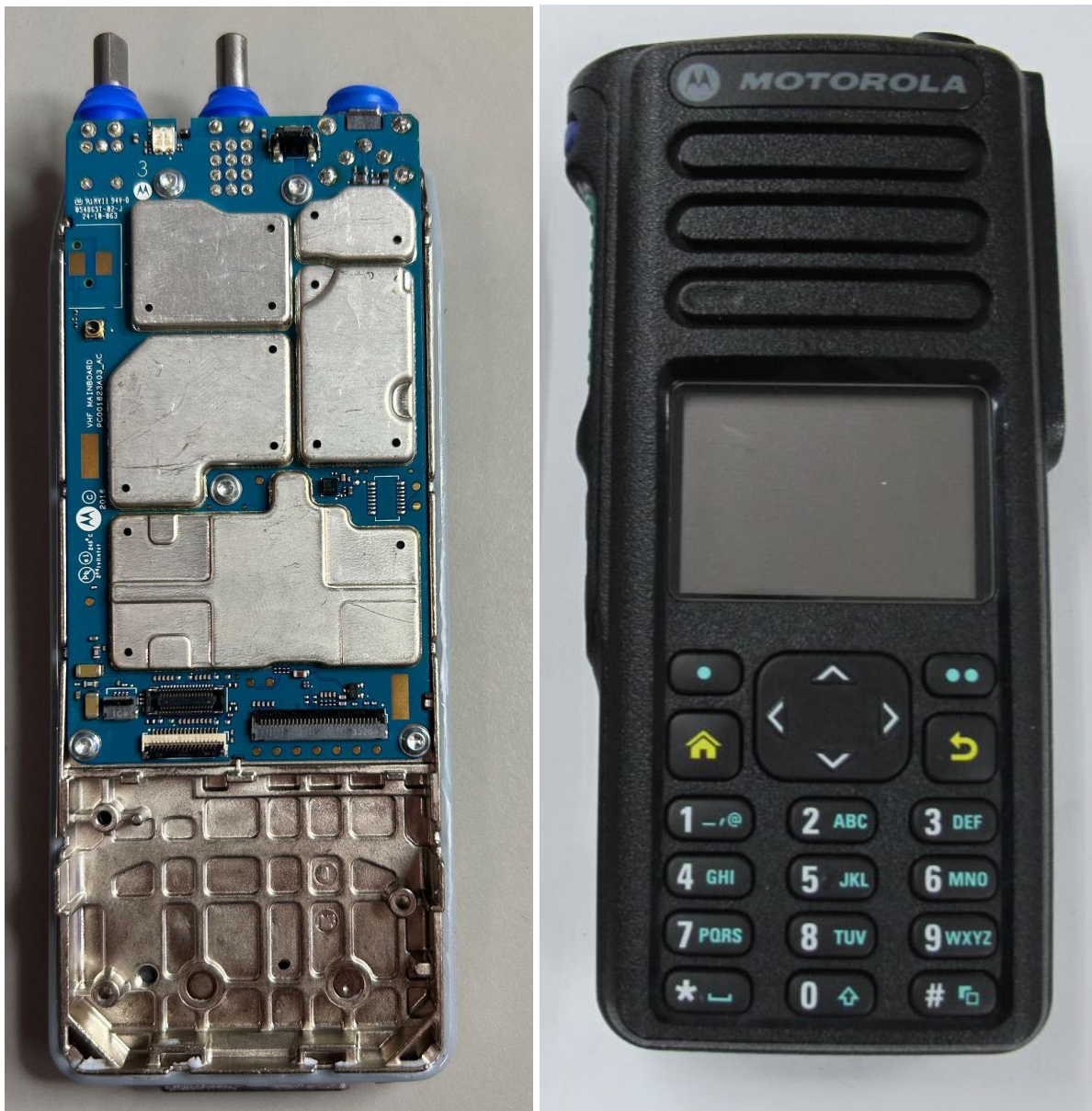
RF board with chasis and housing (front) Model 3 (APX900)
