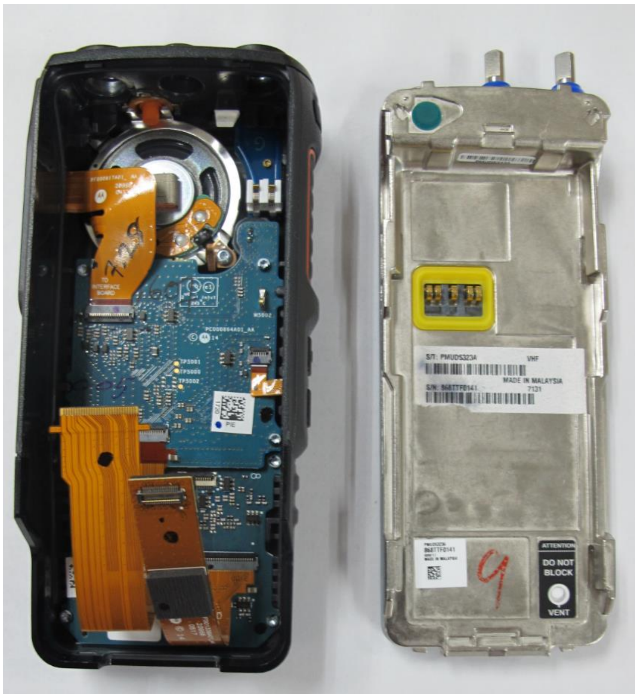
Chassis and Housing (Back), Model 3 (VX-P949)
