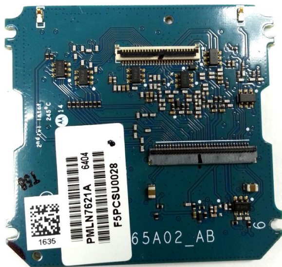
Keypad board (Bottom), Model 3 (VX-P949)
