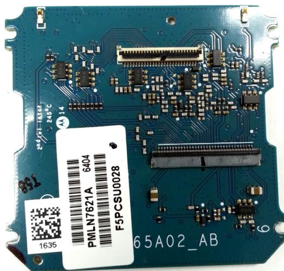
Keypad board (Bottom), Model 3 (APX900)
