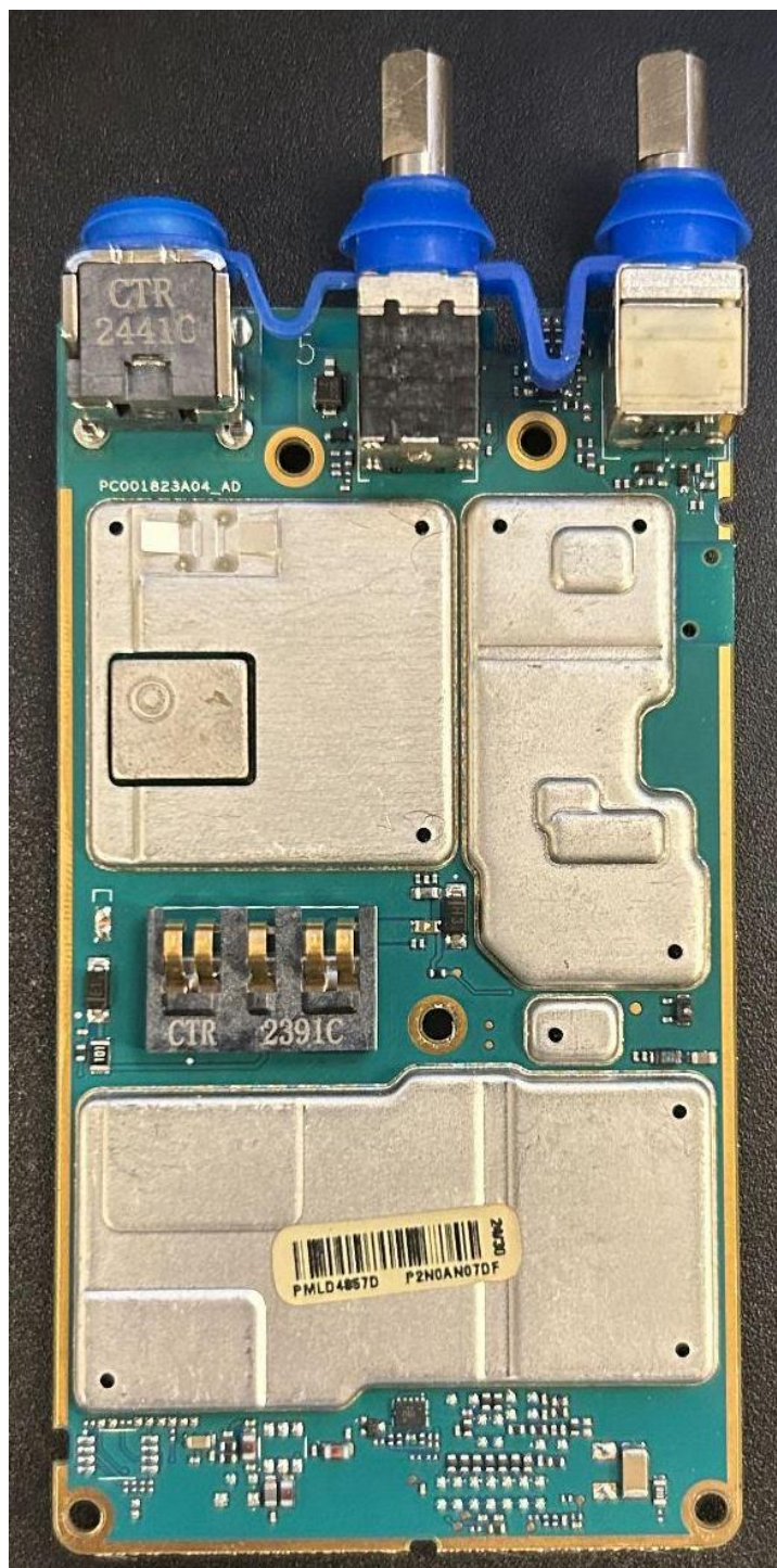
RF board with Shields (Bottom) (APX900 & VX-P949)
