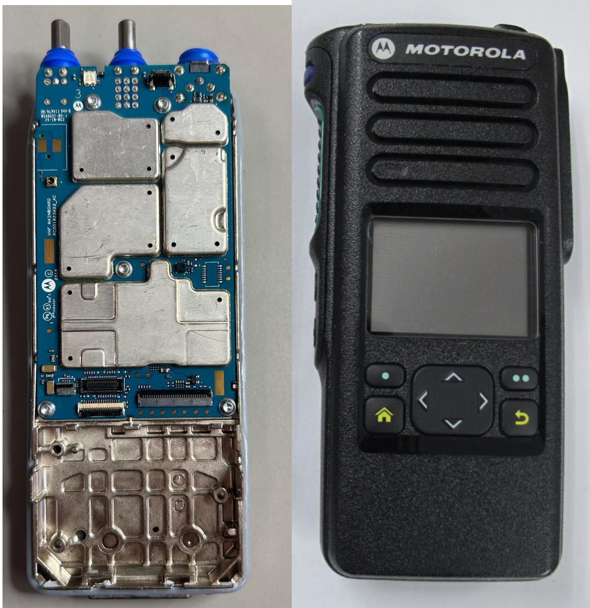
RF board with chassis and housing (front) Model 2 (APX900)
