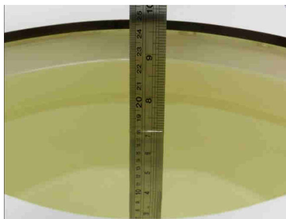
Fig 10.2 Photo of Liquid Height for Body SAR
