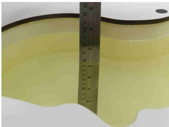
Fig 10.1 Photo of Liquid Height for Head SAR
