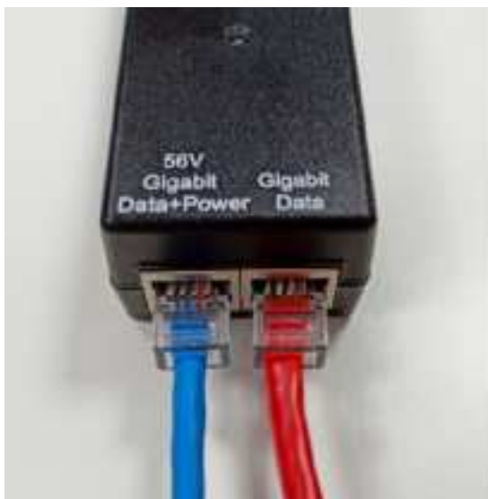
Figure 128: Connecting the V1000 power injector
