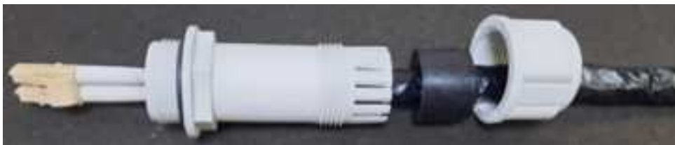
Figure 131: Threading the part onto the cable
