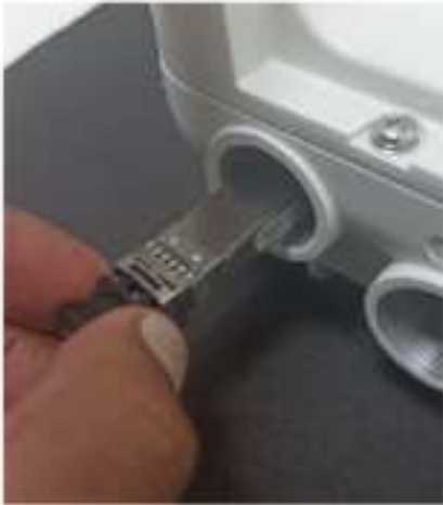
Figure 135: Pushing the module home
