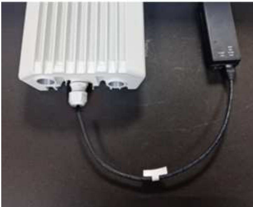
Figure 120: Connecting the power injector to ODU drop cable
