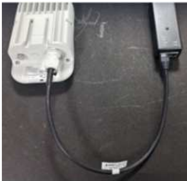
Figure 128: Connecting the V1000 power injector
