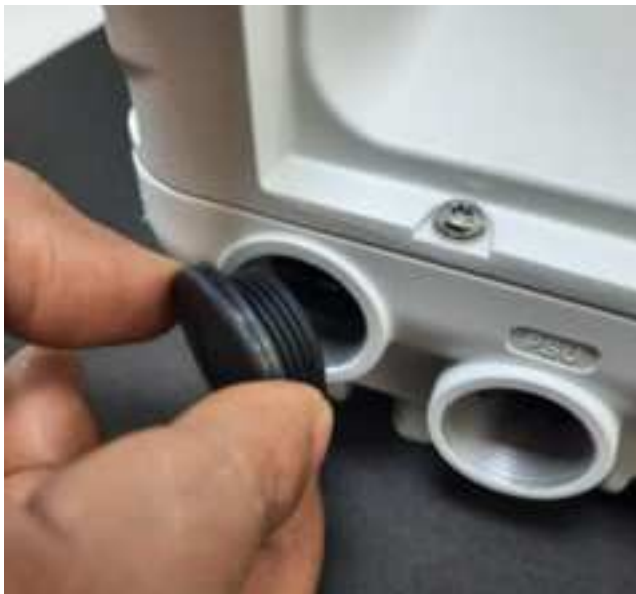
Figure 133: Removing the blanking plug from the SFP port
