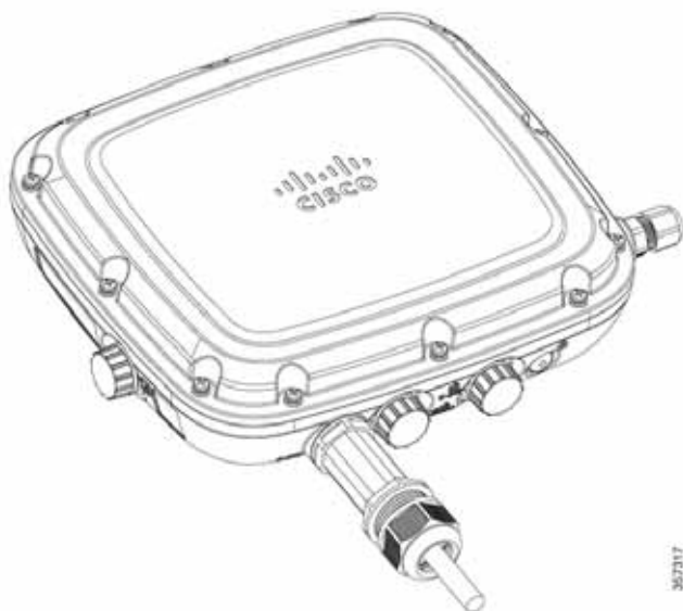
Figure 82: Fiber-Optic cable and gland installed to AP
